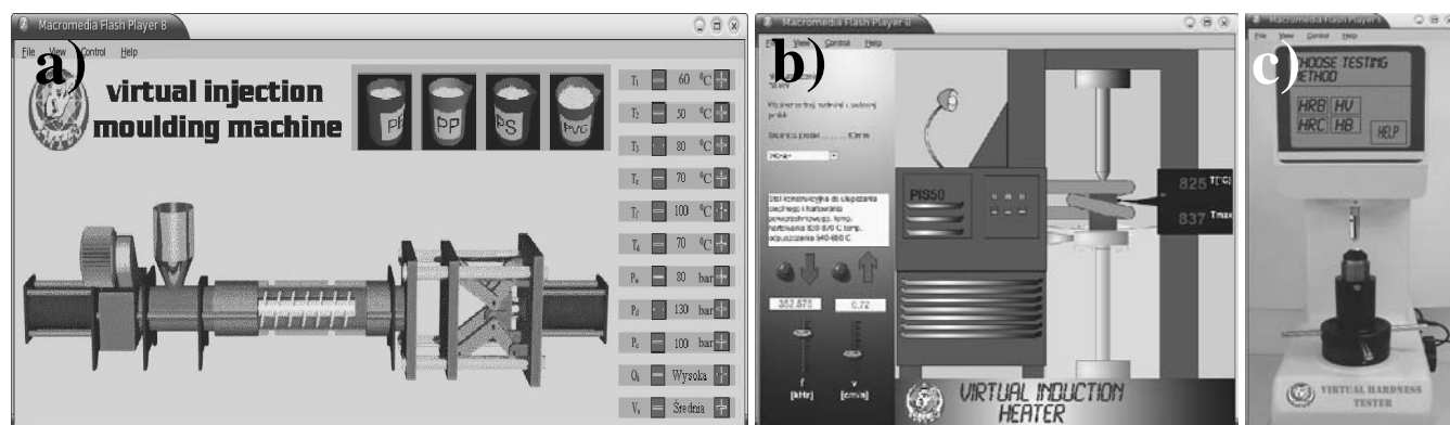
Fig. 2. Examples of virtual devices, which are simulating real scientific equipment a) simulation of injection moulding machine, presented is the the panel for polymer and process parameters selection, b) surface hardening heater PIS50, presented is the heating stage, c) simulation of hardness tester, presented is the panel serving for the choice of the testing method, [6-7,11].
