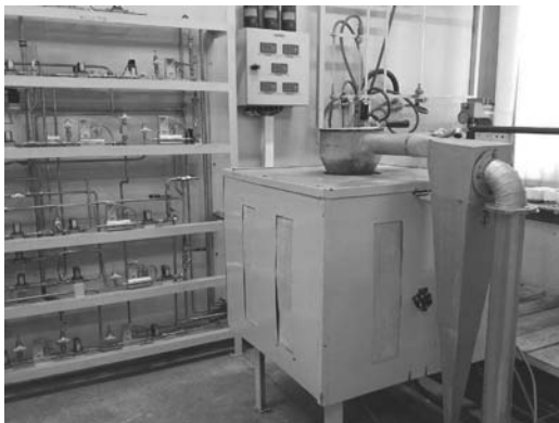
Fig. 2. Fluidized bed and gas distribution station PGIMP-1 [10]
