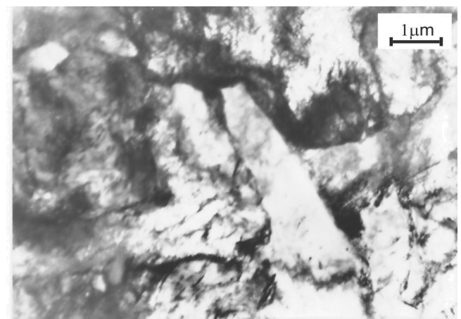
Fig. 10. Structure of the upper bainite with carbide particles on boundaries of particular laths (isothermal holding temperature: 450°C)
