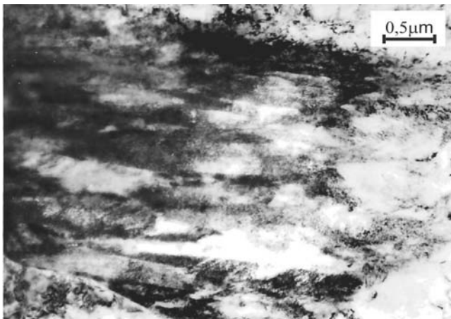
Fig. 7. Retained austenite as films between the laths of the ferritic bainite (isothermal holding temperature: 250°C)
