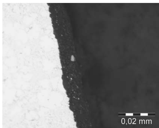
Fig. 17. Oxide cross-sections of anodic layer generated on the EN AC-ALSi12(b) alloy, high pressure cast alloy, light microscope
