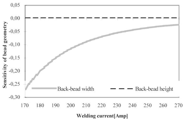
Fig. 4. Sensitivities of bead geometry on welding current
