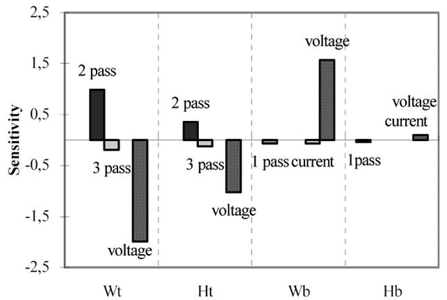
Fig. 1. Bead-geometry sensitivities of process parameters for curvilinear equations
