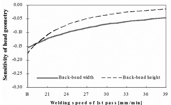
Fig. 3. Sensitivities of bead geometry on 1<sup>st</sup> welding speed
