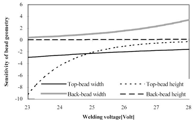
Fig. 2. Sensitivities of bead geometry on welding voltage
