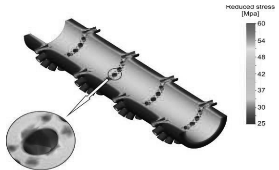
Fig. 7. Distribution of reduced stresses on the chamber inner surface induced by steam's pressure
