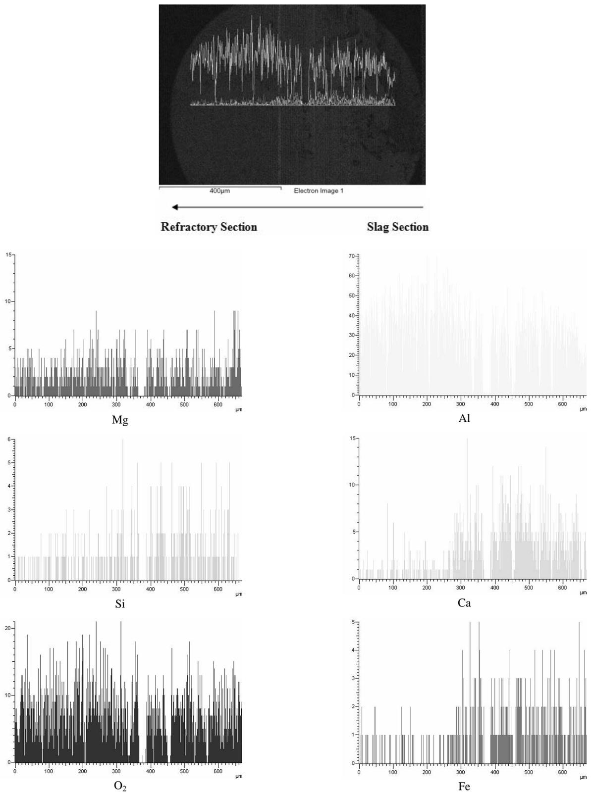
Fig. 10. LineScan analysis of slag penetration layer in castable
