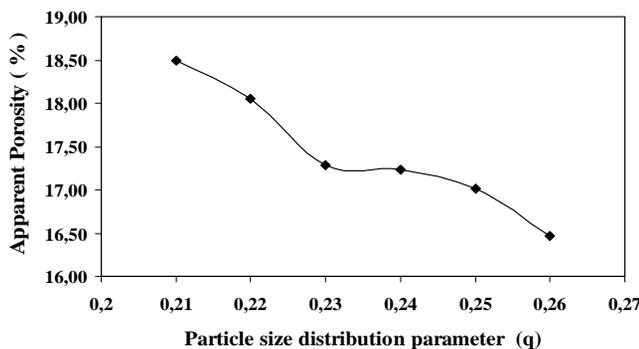
Fig. 4. Apparent porosity as a function of particle size distribution parameter
