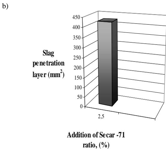
Fig. 7 a-b. Slag penetration areas images (a) and slag penetration areas of castable at 1600°C
