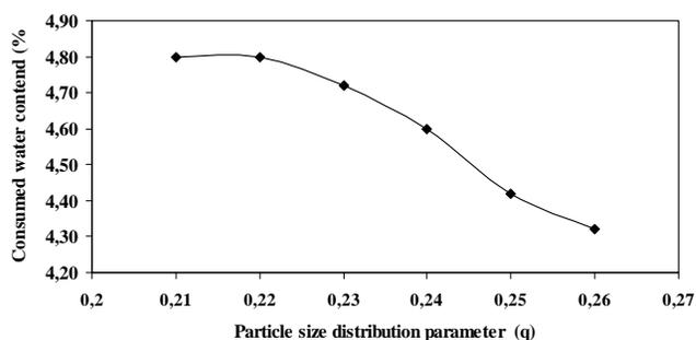
Fig. 2. Water content as a function of particle size distribution parameter
