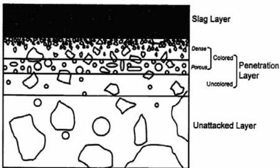
Fig. 8. Schematic diagram of general image of castable after slag corrosion
