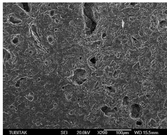
Fig. 9. TEM potomicrograph (20x) of the castable at hot zone
