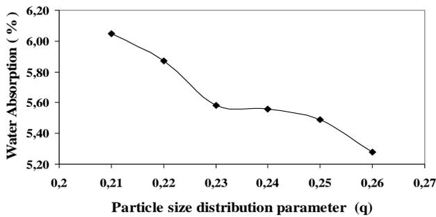
Fig. 3. Water absorption as a function of particle size distribution parameter
