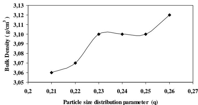
Fig. 5. Bulk density as a function of particle size distribution parameter
