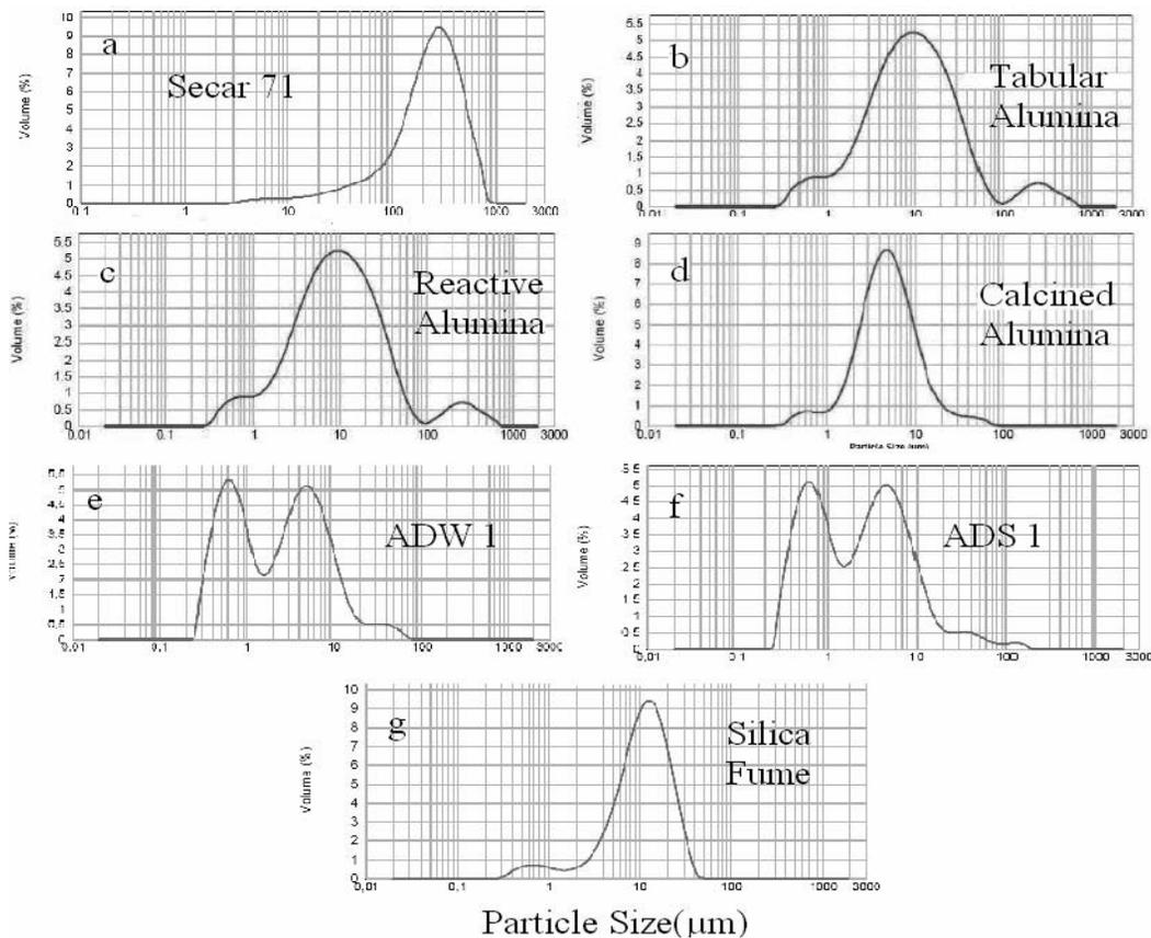
Fig. 1. Particle size distributions of a) secar 71, b) tabular alumina(-0.04 mm), c) reactive alumina, d) calcined alumina, e) ADW1, f) ADS1, g) Micro silica
