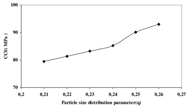
Fig. 6. Cold crushing strength as a function of particle size distribution parameter
