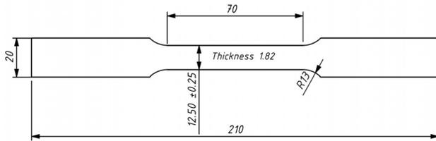
Fig. 1. Tensile test specimens (Dimension are in mm)
