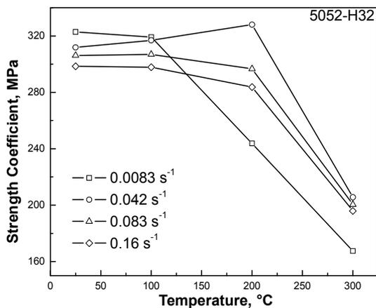
Fig. 6. Strength coefficient versus temperature
