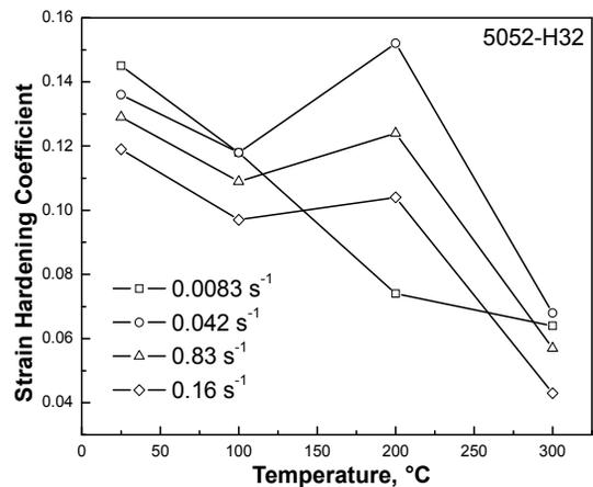
Fig. 5. Strain hardening coefficient (*n*) versus temperature
