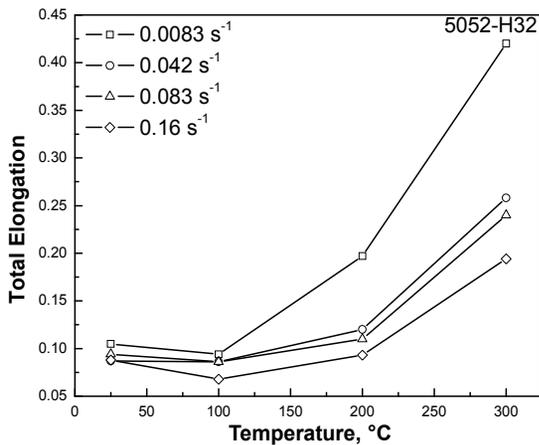
Fig. 3. Total elongation versus temperature
