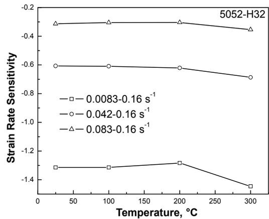
Fig. 4. Strain rate sensitivity versus temperature
