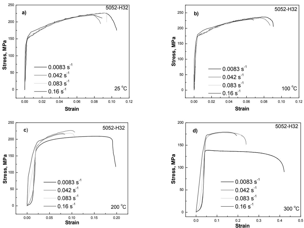
Fig. 2. True stress versus true strain curves at various temperatures and strain rates
