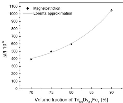
Fig. 5. Measured results for magnetostriction of composites with different volume fractions of  $Tb_{0.3}Dy_{0.7}Fe_{1.9}$ . Measurements were made at  $B = 0.48$  T
