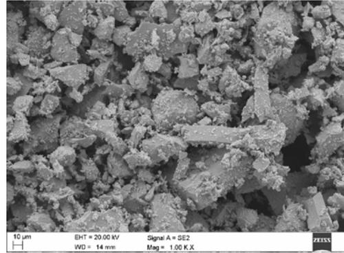
Fig. 1. Morphology of the  $Tb_{0.3}Dy_{0.7}Fe_{1.9}$  powder particles with the average size of 38-106 µm observed by SEM
