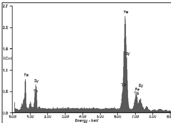
Fig. 3. EDS analysis of the  $Tb_{0.3}Dy_{0.7}Fe_{1.9}$  powder
