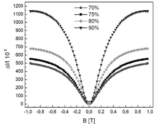
Fig. 4. Effective magnetostriction in the direction of magnetic field vs. applied magnetic field for composites with different volume fraction of  $Tb_{0.3}Dy_{0.7}Fe_{1.9}$
