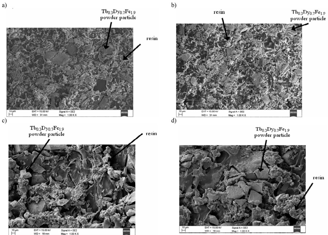
Fig. 2. SEM micrograph of a cross section of composite with 70 % (a), 75 % (b), 80 % (c) and 90 % (d) volume fraction of  $Tb_{0.3}Dy_{0.7}Fe_{1.9}$
