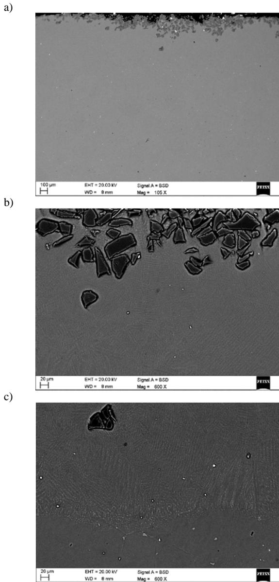
Fig. 4. Scanning electron micrograph laser surface modified MCMgAl3Zn1 with SiC particle a) of the cross-section of the coating, b) top surface of the coating, c) interface between modified zone and the substrate (laser power: 1.6 kW, scan rate: 0.75 m/min, powder feed rate: 8-9 g/min)
