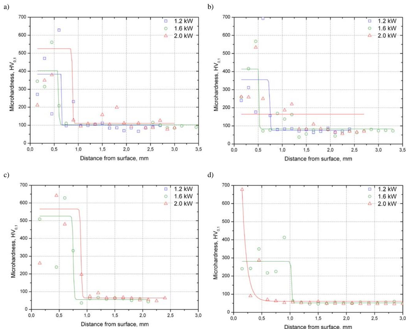
Fig. 8. Cross-section microhardness profile from the surface: a) MCMgAl12Zn1, b) MCMgAl9Zn1, c) MCMgAl6Zn1, d) MCMgAl3Zn1 alloy with SiC particles, scan rate: 0.75 m/min
