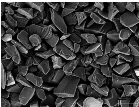
Fig. 1. Morphology of silicon carbide (SEM)
