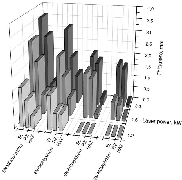
Fig. 2. Diagram of thickness changes of particular areas in the surface layers after alloying SiC powder: SL – surface layer, HAZ – heat affected zone, RZ – remelted zone
