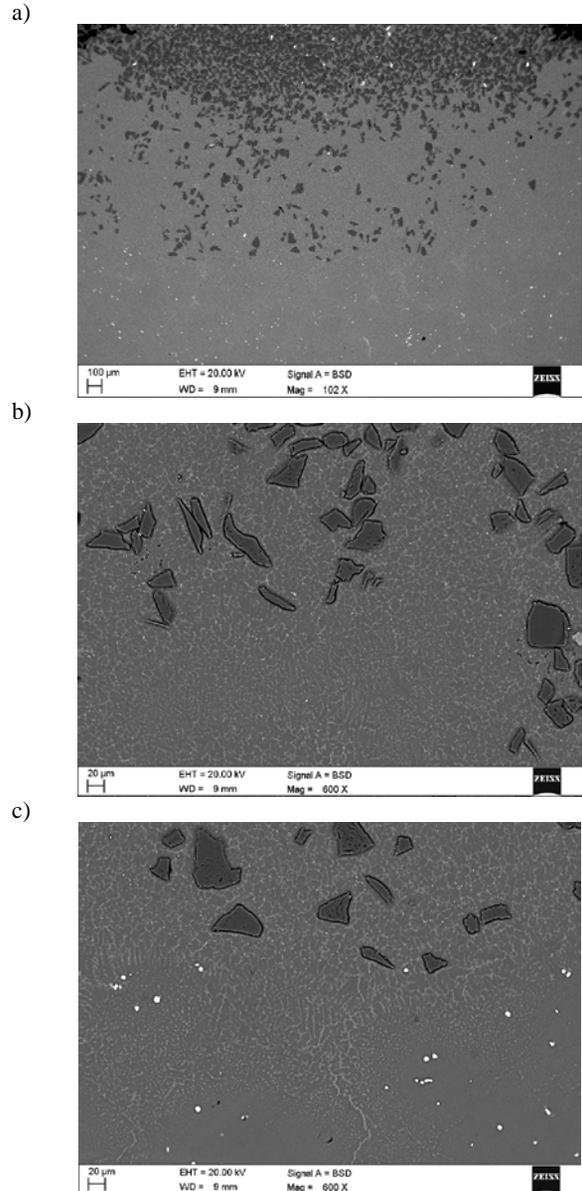
Fig. 3. Scanning electron micrograph laser surface modified MCMgAl9Zn1 with SiC particle a) of the cross-section of the coating, b) top surface of the coating, c) interface between modified zone and the substrate (laser power: 2.0 kW, scan rate: 0.75 m/min, powder feed rate:  $8 \pm 1$  g/min)
