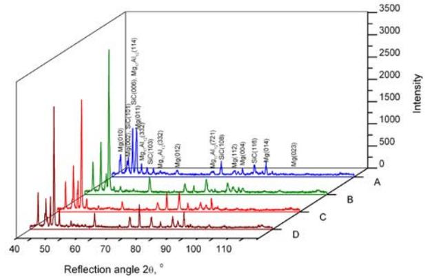
Fig. 5. X ray diffraction pattern of the: A – MCMgAl12Zn1, B - MCMgAl9Zn1, C – MCMgAl6Zn1, D – MCMgAl3Zn1 cast magnesium alloy after laser alloying with SiC: powder feed rate: 8-9 g/min, scan rate: 0.75 m/min, laser power: 2.0 kW
