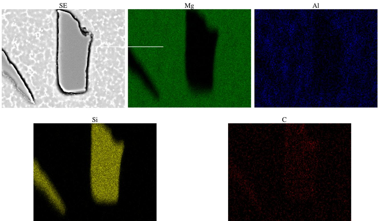
Fig. 7. X-ray mapping of the microstructure MCMgAl9Zn1 alloying layer and the distribution of Mg, Al, Si, C
