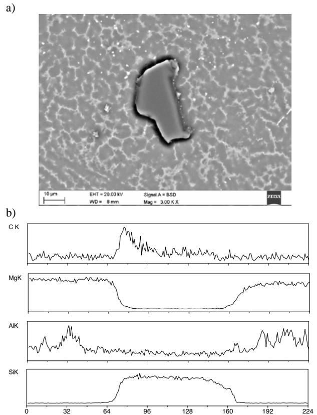
Fig. 6. Scanning electron microscopy micrograph of MCMgAl9Zn1 alloy after laser alloying with SiC particles, laser power: 2.0 kW, scan rate: 0.75 m/min, powder feed rate: 8-9 g/min, a) SEM micrograph, b) linear analysis of the chemical composition changes
