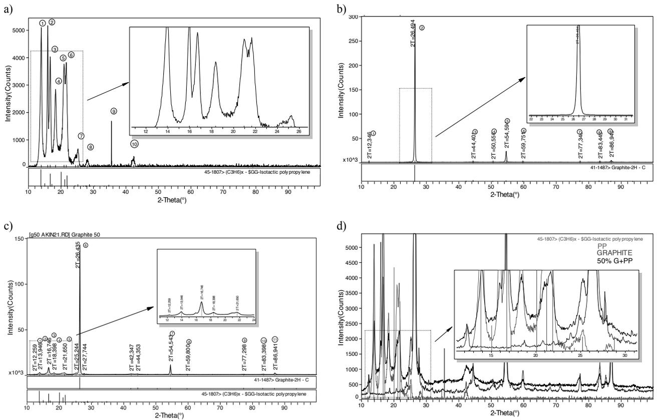
Fig. 1. XRD patterns of the pure iPP (a), graphite (b) and including 10–50 wt. % graphite iPP matrix composites (c), (d)
