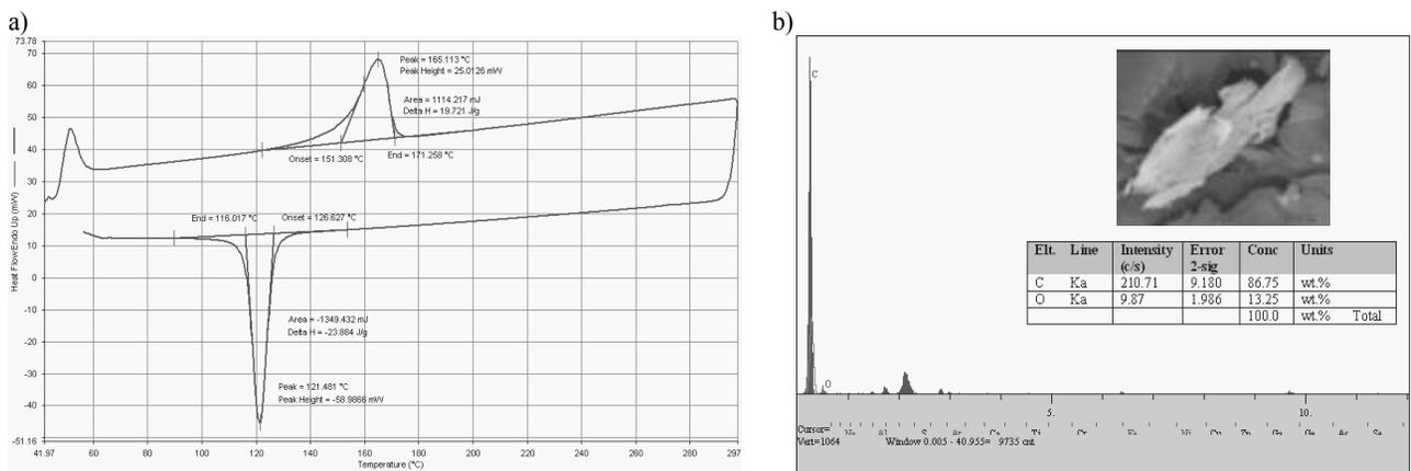
Fig. 2. DSC thermogram (a) and EDS analysis (b) of iPP composite included 50wt. graphite
