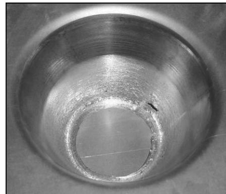
Fig. 11. The cone formed with tool rotation of 40 rpm and dry friction
