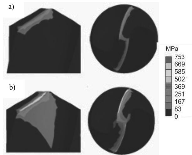
Fig. 16. Example stresses distribution in drill for point angle  $2\kappa_2 = 120^\circ$  made of X39Cr13 steel loaded with the force a)  $F = 100$  N, b)  $F = 200$  N
