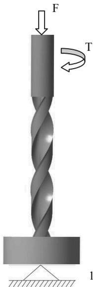
Fig. 5. Numerical model with boundary conditions F- force, T-torque, 1- fixed support
