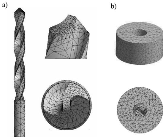
Fig. 3. Meshed model: a – surgical drill, b – disc simulated of bone
