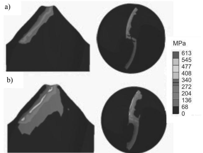
Fig. 9. Example stresses distribution in drill for point angle  $2\kappa_1 = 90^\circ$  made of grade D loaded with the force a)  $F = 100$  N, b)  $F = 200$  N
