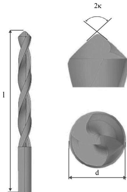
Fig. 1. Geometrical model of the surgical drill
