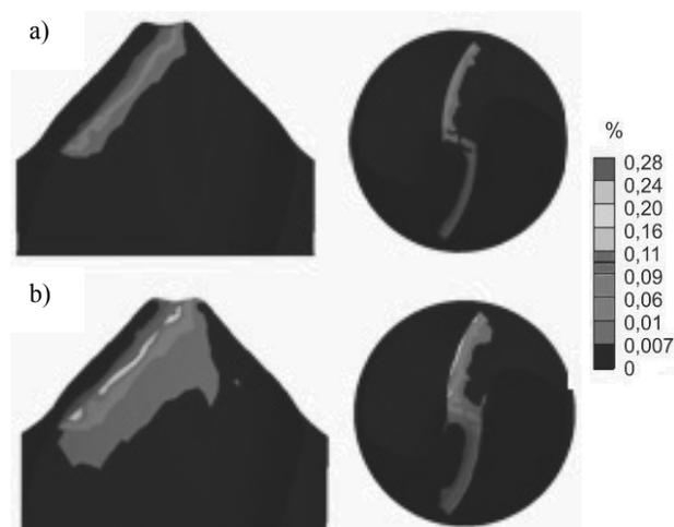
Fig. 12. Example strains distribution in drill for point angle  $2\kappa_1 = 90^\circ$  made of X39Cr13 steel loaded with the force a)  $F = 100 N$ , b)  $F = 200 N$
