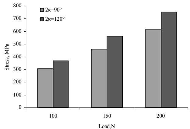
Fig. 17. Relation maximum reduced stresses drills point as a function of the applied loading
