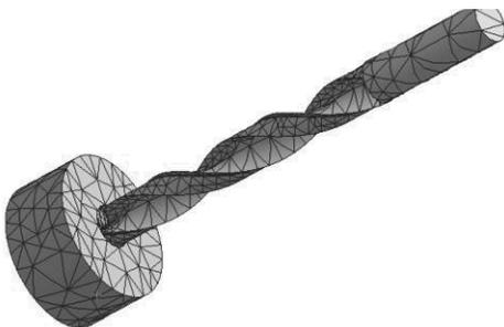
Fig. 4. Meshed model surgical drill – bone system
