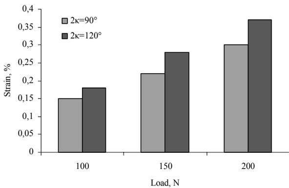
Fig. 8. Relation maximum reduced strains drills point as a function of the applied loading
