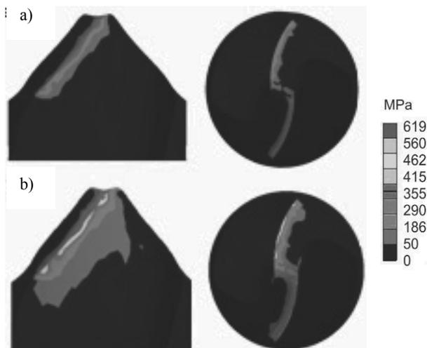
Fig. 15. Example stresses distribution in drill for point angle  $2\kappa_1 = 90^\circ$  made of X39Cr13 steel loaded with the force a)  $F = 100$  N, b)  $F = 200$  N
