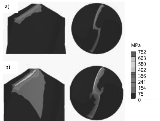
Fig. 10. Example stresses distribution in drill for point angle  $2\kappa_2 = 120^\circ$  made of grade D loaded with the force a)  $F = 100$  N, b)  $F = 200$  N
