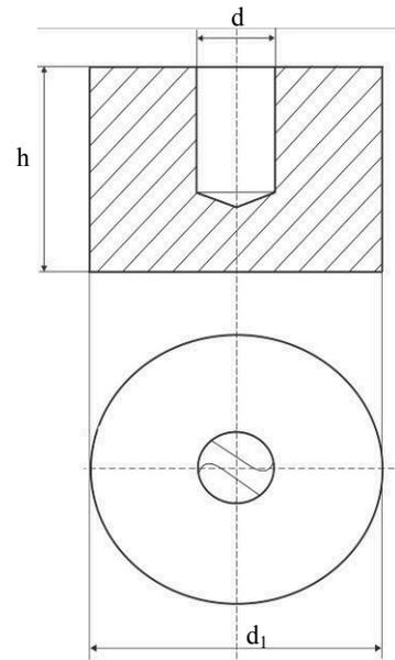
Fig. 2. Geometrical model of the disc simulated of bone
