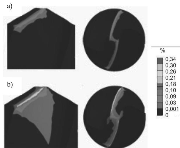
Fig. 13. Example strains distribution in drill for point angle  $2\kappa_2 = 120^\circ$  made of X39Cr13 steel loaded with the force a)  $F = 100 N$ , b)  $F = 200 N$
