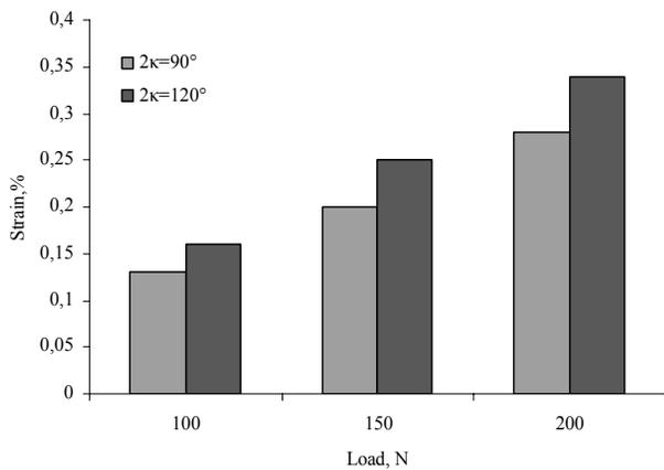
Fig. 14. Relation maximum reduced strains drills point as a function of the applied loading
