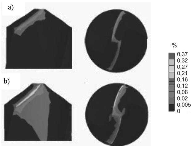
Fig. 7. Example strains distribution in drill for point angle  $2\kappa_2 = 120^\circ$  made of grade D loaded with the force a)  $F = 100$  N, b)  $F = 200$  N
