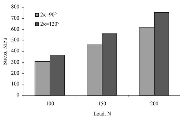
Fig. 11. Relation maximum reduced stresses drills point as a function of the applied loading
