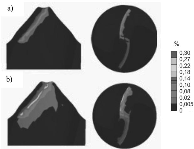
Fig. 6. Example strains distribution in drill for point angle  $2\kappa_1 = 90^\circ$  made of grade D loaded with the force a)  $F = 100$  N, b)  $F = 200$  N
