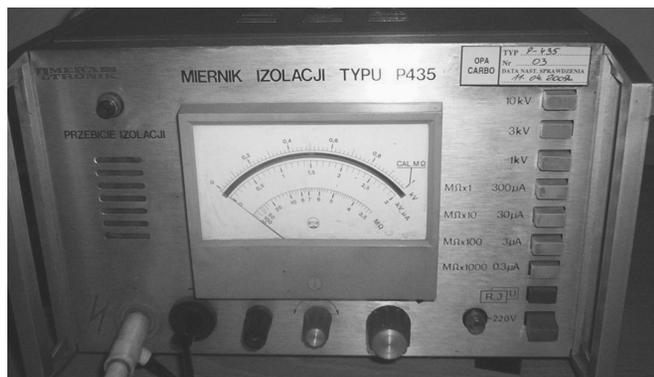
Fig. 5. Insulation Resistance Tester Type P435
