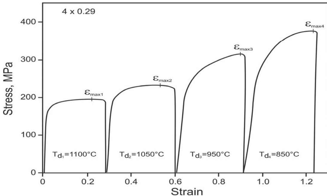
Fig. 5. Stress - strain curves after the multi-stage compression test of the axisymmetrical specimens deformed with a true strain  $4 \times 0.29$  in a temperature range from 1100 to 850°C
