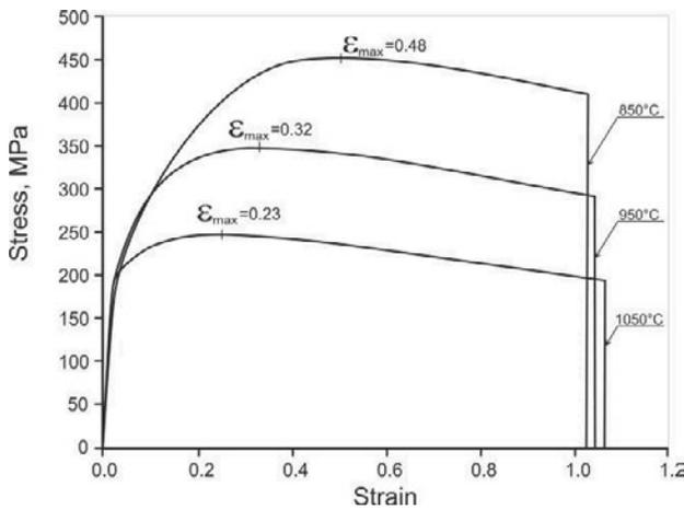
Fig. 4. Influence of the temperature on a shape of  $\sigma$ - $\epsilon$  curves for the specimens compressed with a strain rate of  $10s^{-1}$
