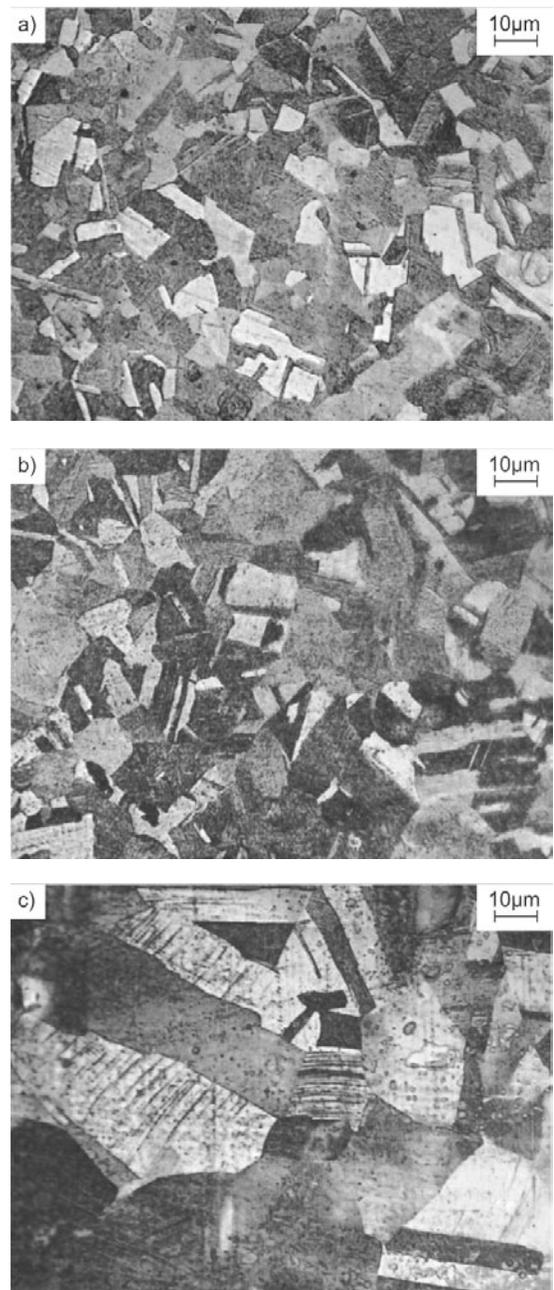
Fig. 3. Austenitic structures of the steel after solution heat treatment from a temperature: a)  $900^{\circ}C$ , b)  $1000^{\circ}C$ , c)  $1100^{\circ}C$
