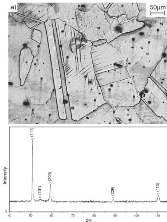
Fig. 2. Austenitic structure with annealing twins and  $\epsilon$  martensite plates of the 27Mn-4Si-2Al-Nb-Ti steel in the initial state (a) and X-ray diffraction pattern (b)
