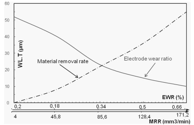
Fig. 3. The influence of the material removal rate  $MRR$  and the electrode wear ratio  $EWR$  on the thickness of the white layer
