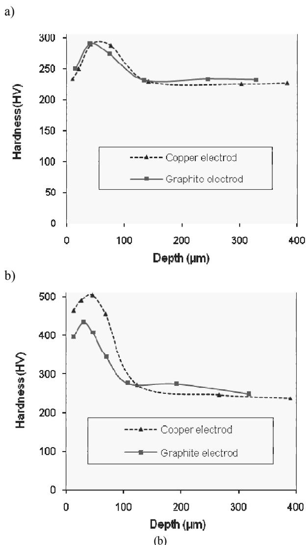
Fig. 8. The influence of the tool material on the evolution of the hardness profile; (a) Completion of machining, (b) Roughing machining
