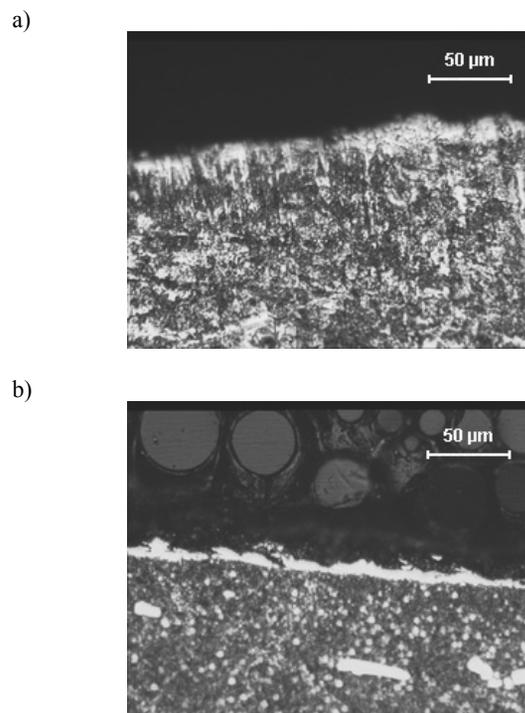
Fig. 6. Comparison between two surfaces machined by: (a) EDM, WLT = 3.75 $\mu\text{m}$  and (b) WEDM, WLT = 3.15 $\mu\text{m}$
