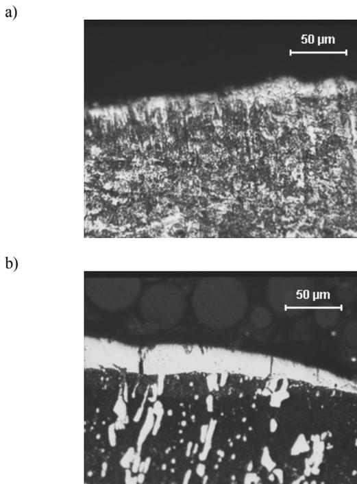
Fig. 5. Comparison between the white layer thicknesses of two different work piece material in half completion EDM; (a) 50CrV4: WLT = 18.7 $\mu\text{m}$ , (b) X200Cr15: WLT = 17.76  $\mu\text{m}$
