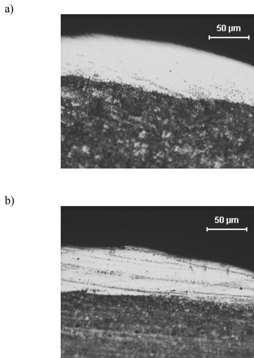
Fig. 4. Influence of the tool material on the white layer thickness WLT in roughing EDM; (a) Copper electrode  $WLT = 53.65$   $\mu\text{m}$ , (b) graphite electrode  $WLT = 51.88$   $\mu\text{m}$
