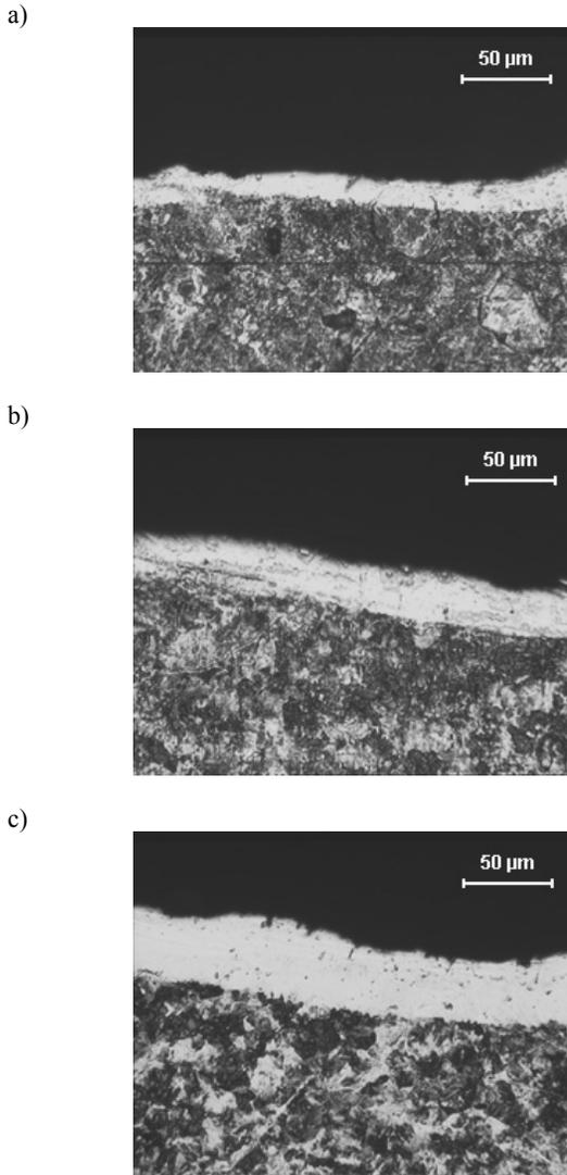
Fig. 2. Analyse of the White Layer Thickness WLT as a function of the machined energy  $W$  observed under an optical microscope; (a)  $W = 38.4$  J,  $WLT = 13.7\mu\text{m}$ ; (b)  $W = 99.84$  J,  $WLT = 18.7\mu\text{m}$ ; (c)  $W = 384$  J,  $WLT = 31.95\mu\text{m}$
