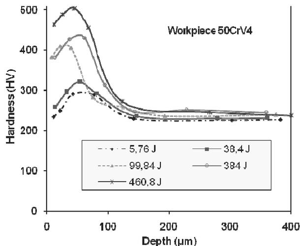
Fig. 7. The influence of the discharge energy on the depth hardness profile
