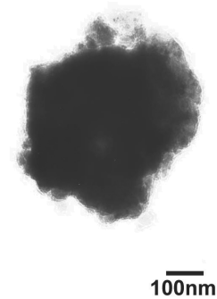
Fig. 14. TEM image of Ti_7Si_2C alloy after 200hrs of mechanical alloying
