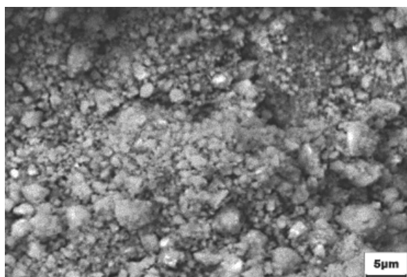
Fig. 6. Structure of powder's mixture of Ti_7Si_2C alloy after 200hrs of mechanical alloying (SEM, 2400x)
