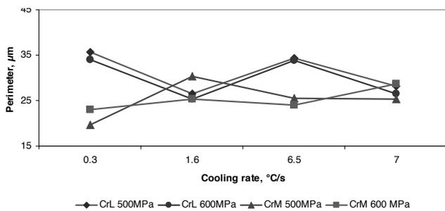
Fig. 17. The average values of pores' perimeter existed in sintered steel based on pre-alloyed Astaloy CrL and Astaloy CrM powders
