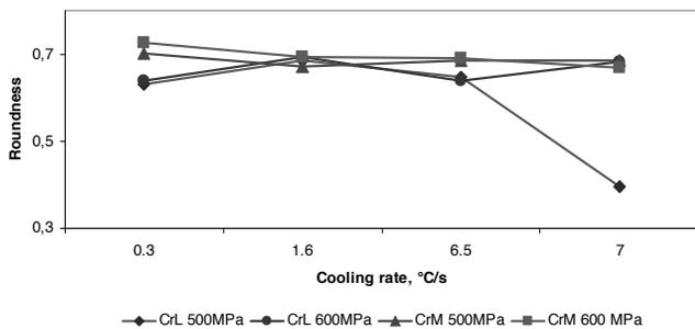
Fig. 18. The mean values of pores' roundness existed in sintered steel based on pre-alloyed Astaloy CrL and Astaloy CrM powders
