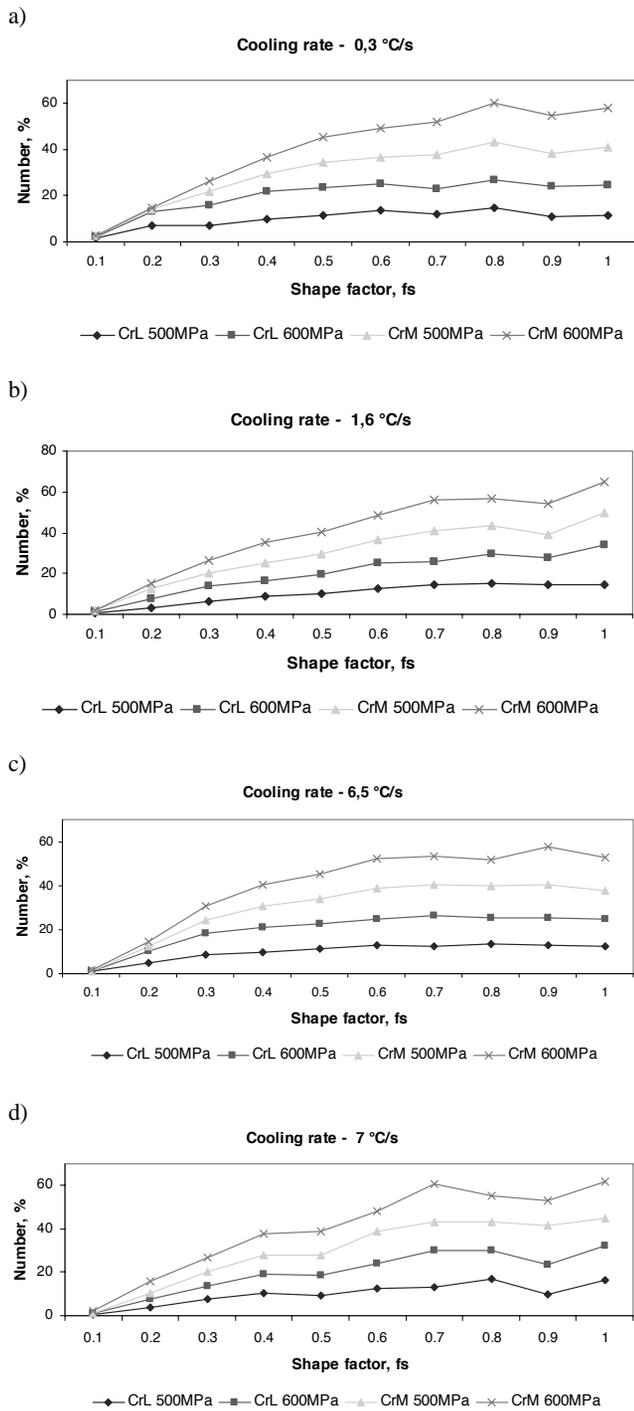
Fig. 13. Influence of four cooling rates: a) slow cooling (0.3°C/s), b) medium cooling (1.6°C/s), c) rapid cooling (6.5°C/s), d) rapid cooling (7°C/s) on distribution of the dimensionless shape factor - fs
