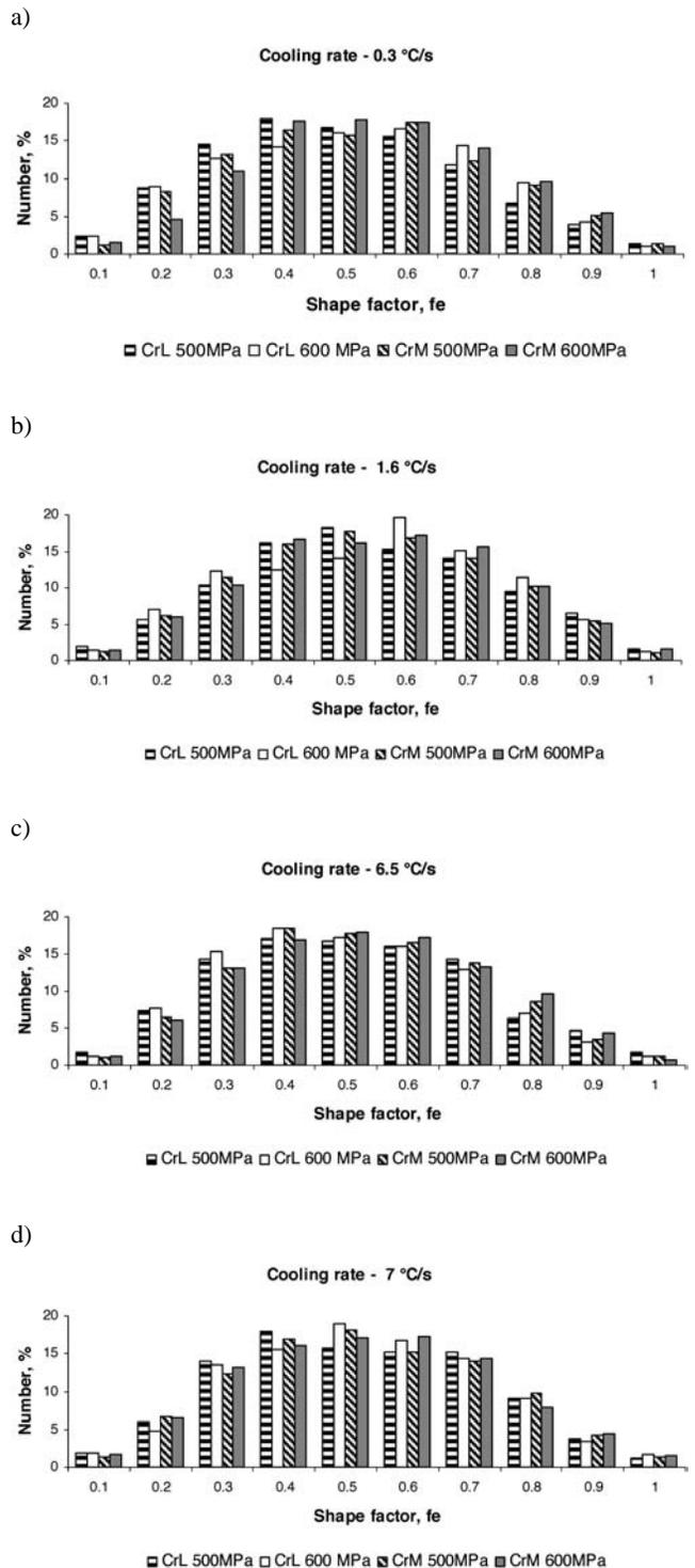
Fig. 12. Influence of four cooling rates: a) slow cooling (0.3°C/s), b) medium cooling (1.6°C/s), c) rapid cooling (6.5°C/s), d) rapid cooling (7°C/s) on distribution of the dimensionless shape factor -  $f_e$
