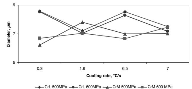
Fig. 15. The average values of pores' diameter existed in sintered steel based on pre-alloyed Astaloy CrL and Astaloy CrM powders
