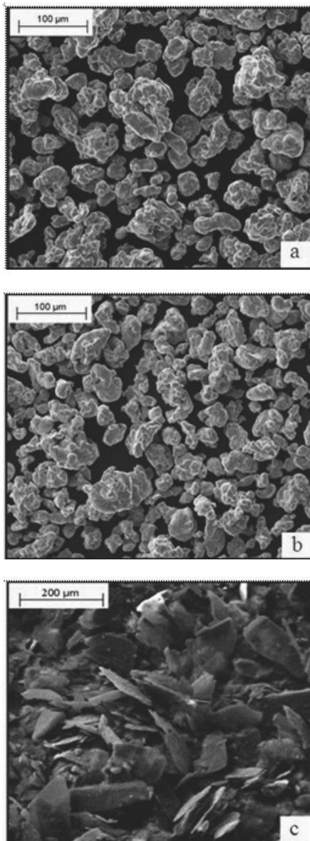
Fig. 4. Micrographs of base powders: a) Astaloy CrL pre-alloyed powder. b) Astaloy CrM pre-alloyed powder. c) GR12 graphite powder (SEM)
