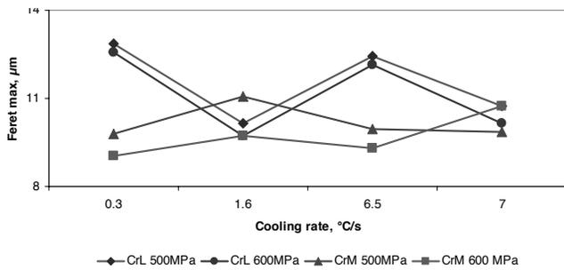
Fig. 16. The average values of pores' Feret max existed in sintered steel based on pre-alloyed Astaloy CrL and Astaloy CrM powders
