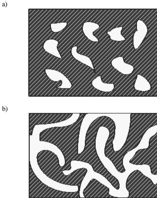
Fig. 1. Diagram of sinter structure with porosity: a) closed; b) open [2]
