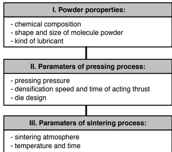
Fig. 3. Factors influence on sinters porosity [1]
