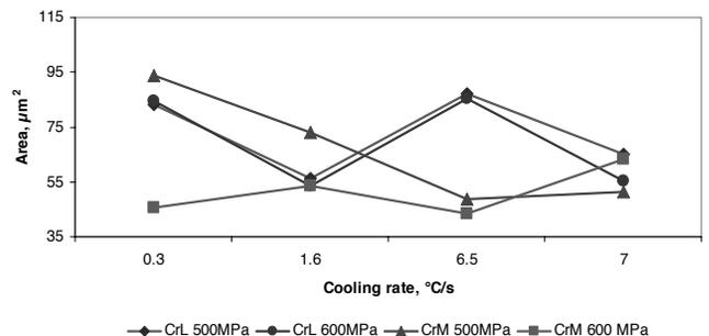
Fig. 14. The average values of pores' area in sintered steel based on pre-alloyed Astaloy CrL and Astaloy CrM powders
