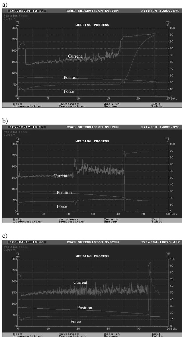
Fig. 7. Welding parameter waveforms of the flash butt welding: a) waveform of the test No 1, b) waveform of the test No 8, c) waveform of the test No 5
