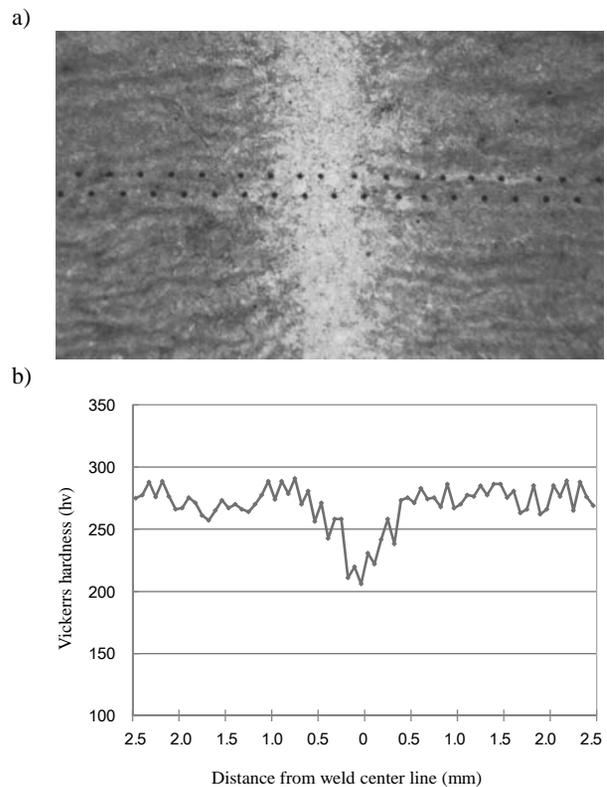
Fig. 6. Micro Vickers hardness test result: a) microstructure of the weld, b) hardness test result
