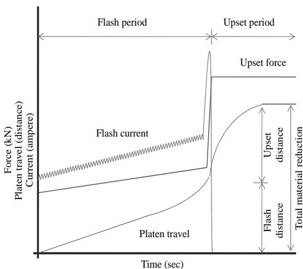
Fig. 1. Schematic of typical flash butt welding process
