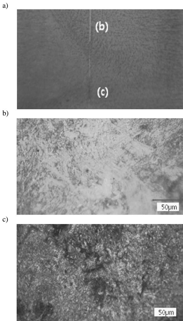
Fig. 5. Macrosection and microstructure of test No. 8: a) macrosection of the weld, b) microstructure of the white line (x50), c) microstructure of the black line (x50)
