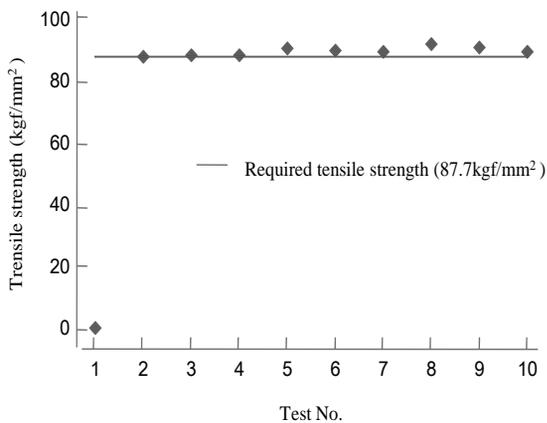
Fig. 3. Tensile strength test result
