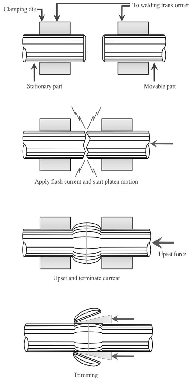
Fig. 2. Basic steps in flash butt welding
