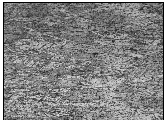
Fig. 7. Structure of copper alloy CB4 with grains of \alpha phase and numerous precipitates, in delivery state; Mag. 1000x
