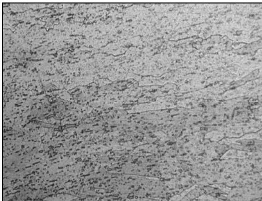
Fig. 9. Structure of copper alloy CCNB with grains of \alpha phase and numerous precipitates in delivery state; Mag. 500x
