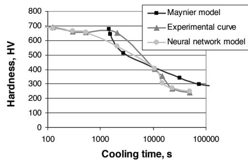
Fig. 4. Comparison of the calculated hardness change curves as function of cooling time with the experimental one for steels austenitised at 860°C with concentrations of: 0.46% C, 0.77% Mn, 0.23% Si, 1.13% Cr, 1.49% Ni, 0.28% Mo, 0.18% V
