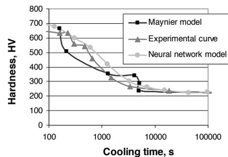
Fig. 5. Comparison of the calculated hardness change curves as function of cooling time with the experimental one for steels austenitised at 880°C with concentrations of: 0.43% C, 0.82% Mn, 0.41% Si, 1.22% Cr, 0.04% Ni, 0.11% V
