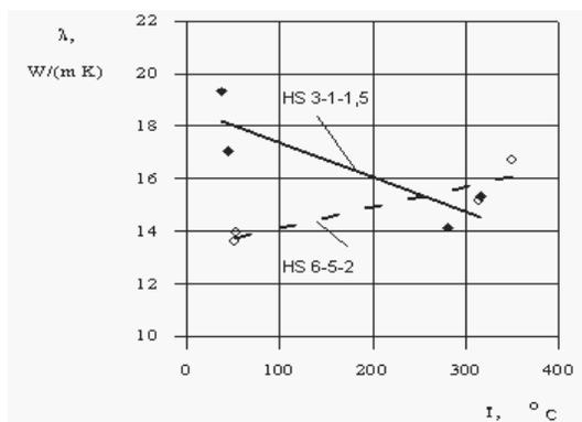
Fig. 2. Relationship between  $\lambda$  coefficient for HS 6-5-2 and HS 3-1-1,5 and measurement temperature
