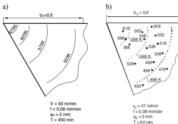
Fig. 1. Thermal field in cutting edge made of a) HS 6-5-2 and b) HS 3-1-1,5 during turning of steel 60 [8,11]
