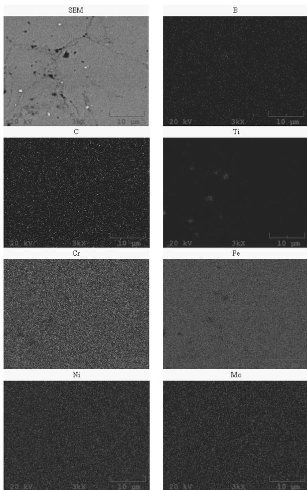
Fig. 4. The SEM microstructure and EDS surface analysis of the AISI 316L stainless steel reinforced with 1% vol.  $\text{TiB}_2$  after sintering at temperature of  $1300^\circ\text{C}$ , at pressure 7.5 GPa
