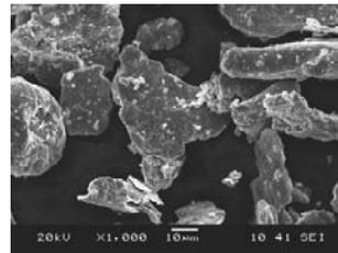
Fig. 1. Morphology of powder particles at magnification 1000x (SEM): a) 316 L steel powder, b)  $\text{TiB}_2$  powder and c) mixture of AISI 316L steel powder and  $\text{TiB}_2$  powder
