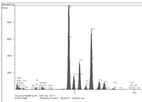
Fig. 3. a) Microstructure of the AISI 316L stainless steel reinforced with 1% vol. TiB<sub>2</sub> (SEM) after sintering at temperature of 1300°C, at pressure 7.5 GPa and b) EDS analysis obtained from point 1
