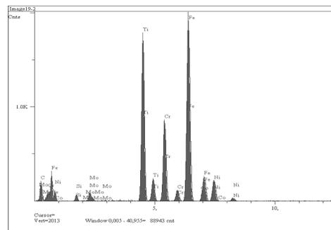
Fig. 2. a) Microstructure of the AISI 316L stainless steel reinforced with 1% vol. TiB<sub>2</sub> (SEM) after sintering at temperature of 900°C, at pressure 7.5 GPa and b) EDS analysis obtained from point 1
