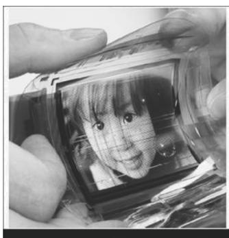
Fig. 6. Photograph of the flexible AMOLED display driven by pentacene TFTs
