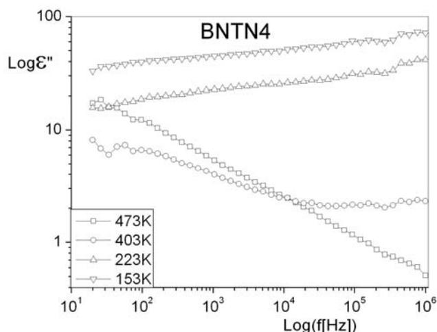
Fig. 3. The dependence of dielectric energy losses on frequency for BNTN4 at selected constant temperatures
