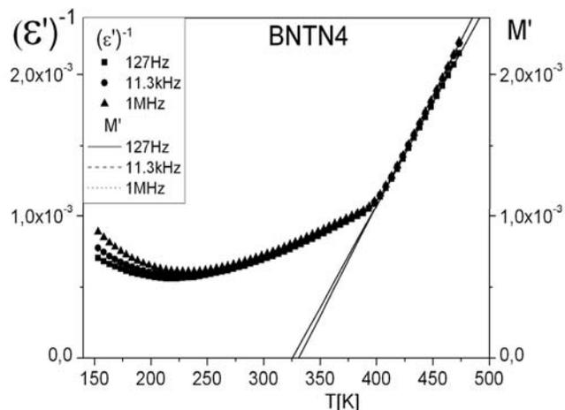
Fig. 5. The inverse of real part of permittivity ( $1/\epsilon'$ ) and real part of electric modulus ( $M'$ ) as a functions of temperature at chosen frequencies for BNTN4 sample
