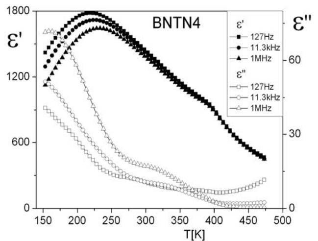
Fig. 1. The dependence of real ( $\epsilon'$ ) and imaginary ( $\epsilon''$ ) parts of dielectric permittivity on temperature and frequency for BNTN4
