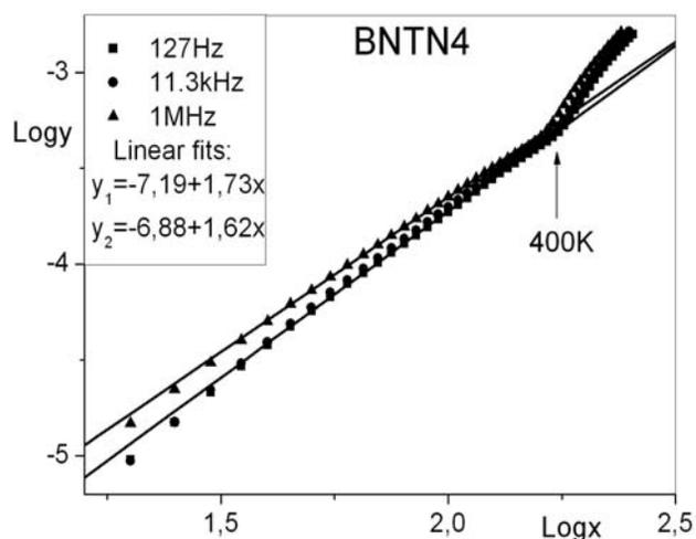
Fig. 6. The dependence of  $\log(y)$  on  $\log(x)$  for BNTN4 sample (for abbreviations see text)
