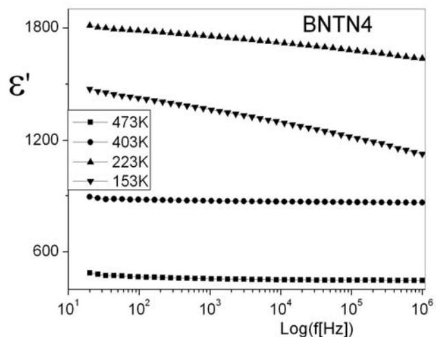
Fig. 2. The dependence of real part of permittivity ( $\epsilon'$ ) on frequency for BNTN4 at selected constant temperatures
