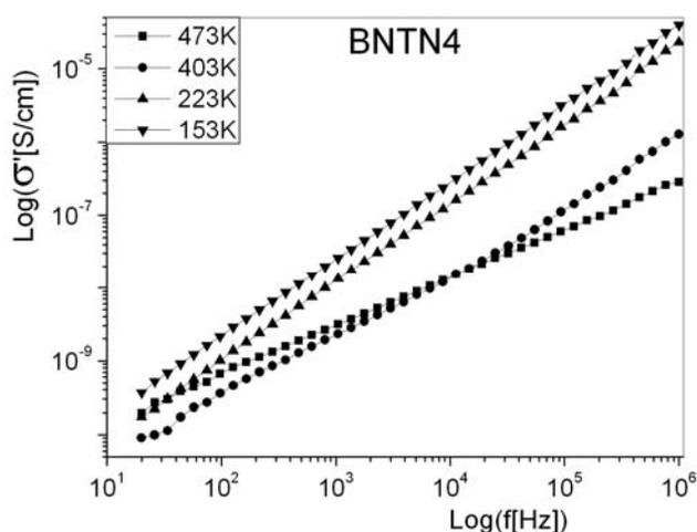
Fig. 4. The dependence of real part of ac conductivity ( $\sigma'$ ) on frequency for BNTN4 at selected constant temperatures
