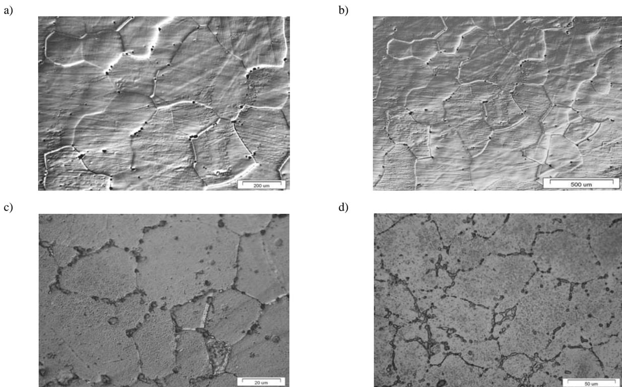
Fig. 2. Microstructure of alloys Ni<sub>3</sub>AlBZr (light microscope): a) alloy A, b) alloy B as cast, c) alloy A, d) alloy B after homogenization
