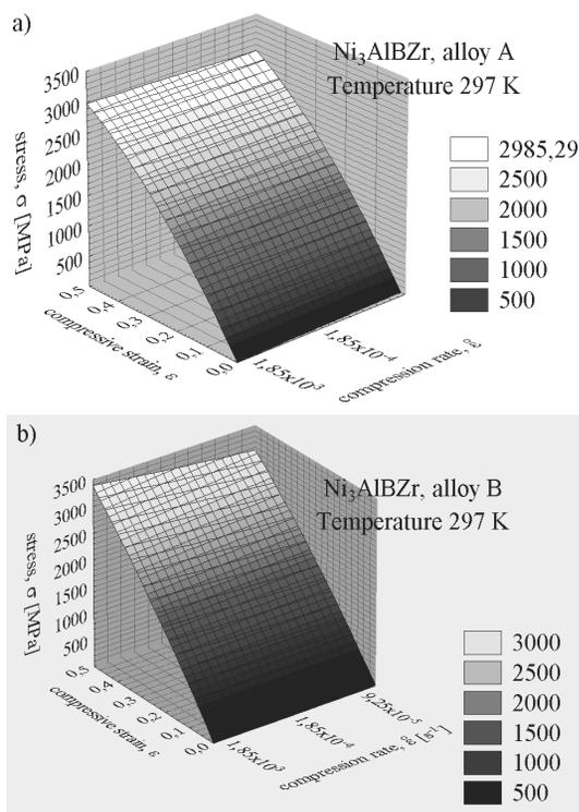
Fig. 4. Mechanical properties of the samples deformations from alloy A and B obtained in the compression tests
