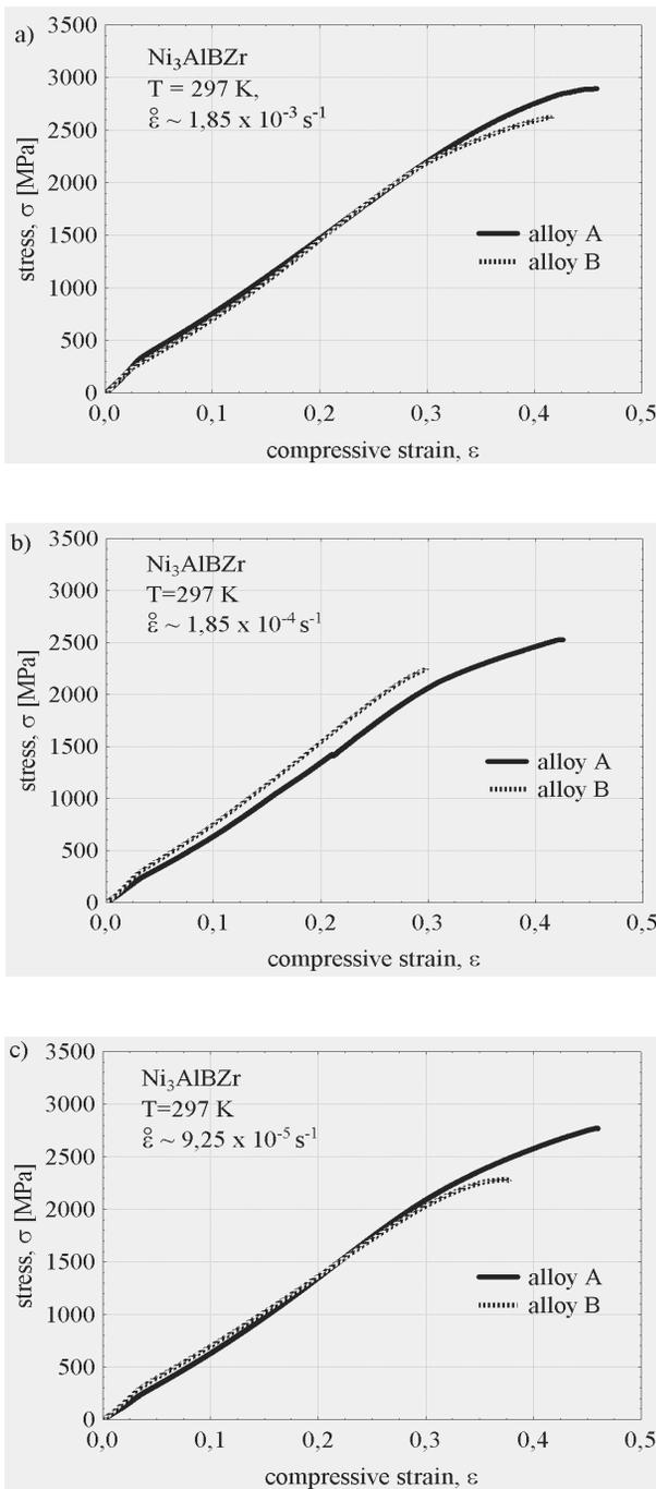
Fig. 3. Flow curves  $\sigma = f(\epsilon)$  for alloys A and B determined in compression tests conducted at strain rate a)  $1.85 \times 10^{-3} \text{ s}^{-1}$ , b)  $1.85 \times 10^{-4} \text{ s}^{-1}$ , c)  $9.25 \times 10^{-5} \text{ s}^{-1}$  and constant temperature 297 K
