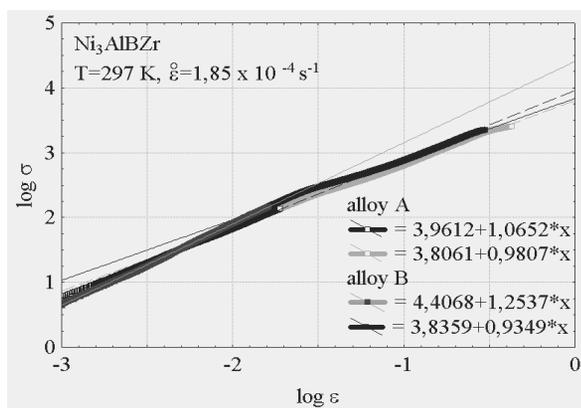
Fig. 5. Strain hardening curves for A and B alloys deformed at a constant temperature and various strain rates
