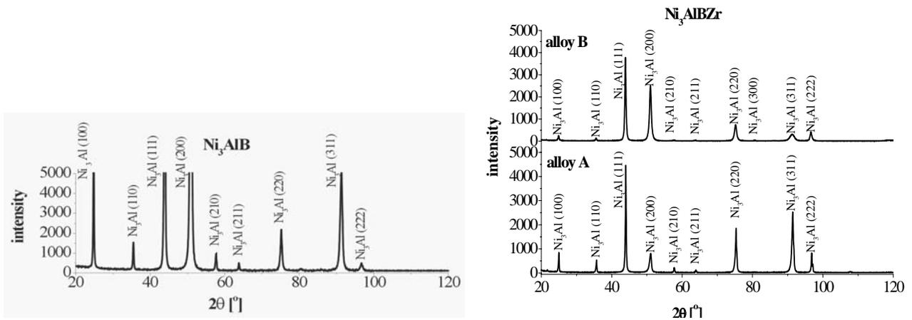
Fig. 1. The diffraction pattern of alloys: Ni<sub>3</sub>AlB as well as Ni<sub>3</sub>AlBZr, alloy A and B, descriptions on drawings
