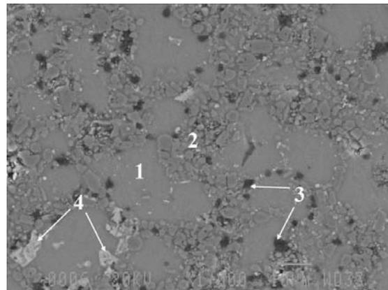
Fig. 9. Microstructure of a TiAl-30 vol. % TiB<sub>2</sub> composite showing different morphologies of the phases observed in the composite: (1) Al<sub>3</sub>Ti grains in TiAl matrix, (2) TiB<sub>2</sub> grains, (3) Al<sub>2</sub>O<sub>3</sub> dark inclusions and (4) traces of Ti<sub>2</sub>Al<sub>5</sub>, TiAl<sub>2</sub>, Ti<sub>5</sub>Al<sub>11</sub> and Ti<sub>9</sub>Al<sub>23</sub>
