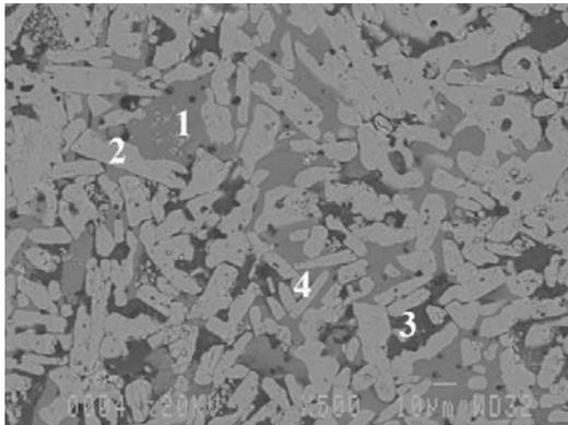
Fig. 15. Individual phases in a fully dense  $\text{Ti}_3\text{Al}$ -40 vol. %  $\text{TiC}$  composite: (1)  $\text{Ti}_3\text{Al}$ , (2)  $\text{Ti-Al-C}$  based grains, (3)  $\text{Ti}_2\text{AlC}$  and (4) Al-based phase
