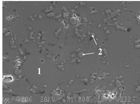
Fig. 8. Scanning electron micrographs of Ti<sub>3</sub>Al-20 vol. % TiB<sub>2</sub> composite showing: (1) Al<sub>3</sub>Ti in sintered Ti<sub>3</sub>Al matrix reinforced with (2) TiB<sub>2</sub> grains
