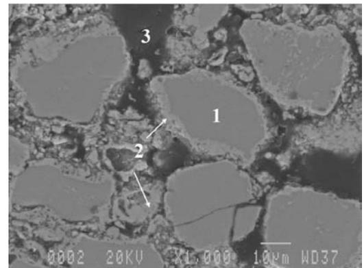
Fig. 5. SEM micrograph of a reactively sintered TiAl-10 vol. % B<sub>4</sub>C composite showing different phases: (1) Al<sub>3</sub>Ti, (2) TiB<sub>2</sub> and (3) Al<sub>2</sub>Ti<sub>4</sub>C<sub>2</sub>
