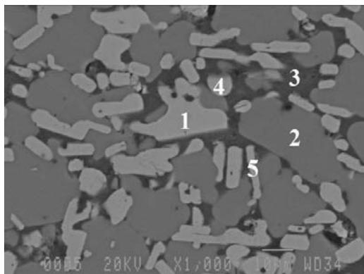
Fig. 12. Individual phases in the microstructure of a  $\text{Ti}_3\text{Al}$ -20 vol.%  $\text{TiC}$  composite: (1)  $\text{Ti-Al}$  phase (2)  $\text{Al}_3\text{Ti}$ , (3) Al-based phase, (4)  $\text{TiC}$  and (5)  $\text{Ti}_2\text{AlC}$
