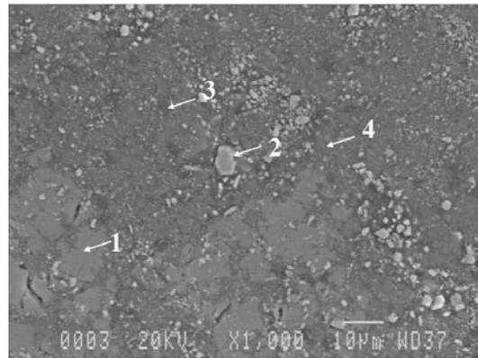
Fig. 4. SEM micrograph of fully dense AlTi-10% B<sub>4</sub>C composite samples with (1) an AlTi alloy matrix (fine and equiaxed  $\gamma$ -TiAl with traces of Ti<sub>2</sub>Al<sub>5</sub>, TiAl<sub>2</sub>, Ti<sub>5</sub>Al<sub>11</sub> and Ti<sub>9</sub>Al<sub>23</sub>), (2) TiB<sub>2</sub> bright grains, (3) TiC gray grains and (4) Al<sub>3</sub>Ti gray phase in the matrix
