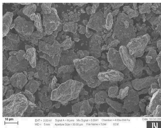
Fig. 3. SEM micrograph of as-received commercial Ti<sub>3</sub>Al powder
