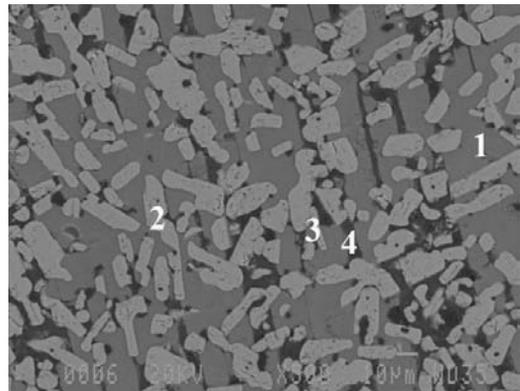
Fig. 13. SEM micrograph of the  $\text{AlTi}$ -30 vol. %  $\text{TiC}$  composite. The individual phases are: (1)  $\gamma$ - $\text{TiAl}$  and  $\alpha_2$ - $\text{Al}_3\text{Ti}$  colonies, (2)  $\text{Ti-Al-C}$  based grains, (3)  $\text{Ti}_3\text{AlC}$  and (4) Al-based phase
