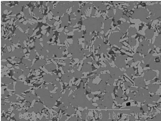
Fig. 11. Microstructure developed in  $\text{Ti}_3\text{Al}$ -20 vol. %  $\text{TiC}$
