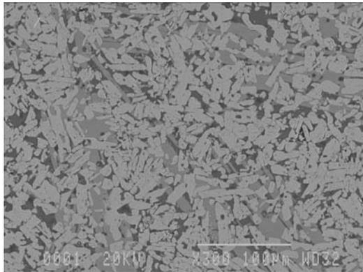
Fig. 14. SEM micrographs of a fully dense  $\text{Ti}_3\text{Al}$ -40 vol. %  $\text{TiC}$  composite
