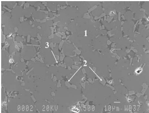
Fig. 10. SEM micrograph of the  $\text{Ti}_3\text{Al}$ -10 vol. %  $\text{TiC}$  composite with: (1)  $\text{Ti}_3\text{Al}$  grains in matrix, (2) a needle-like  $\text{Ti}_3\text{AlC}$  and (3) an Al-based phase
