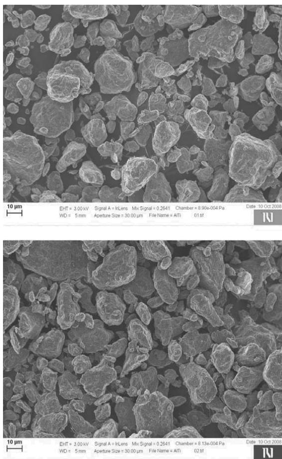
Fig. 2. SEM micrograph of as-received commercial TiAl powder
