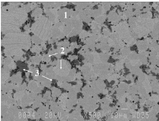
Fig. 7. Microstructure of TiAl-20 vol. %TiB<sub>2</sub> composite. The microstructural constituents are: (1) AlTi lamellae grey phase in the matrix with planar grain boundaries, (2) Ti<sub>3</sub>Al grains in and (3) TiB<sub>2</sub> grains
