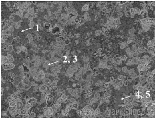
Fig. 6. Representative microstructures of a fully dense Ti<sub>3</sub>Al-40 vol. % B<sub>4</sub>C composite prepared by reactive sintering of Ti<sub>3</sub>Al + 40 vol. % B<sub>4</sub>C: (1) dark spots-B<sub>4</sub>C, (2) and (3) bright phases-AlB<sub>2</sub> and TiB<sub>2</sub>, (4) and (5) grey phases-Al and probably also Al<sub>4</sub>C<sub>3</sub>. In Ti<sub>3</sub>Al matrix, traces of Al<sub>3</sub>BC are also identified
