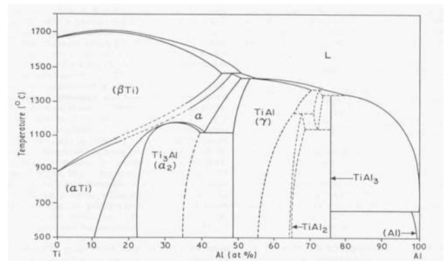
Fig. 1 .Ti-Al phase diagram [20]
