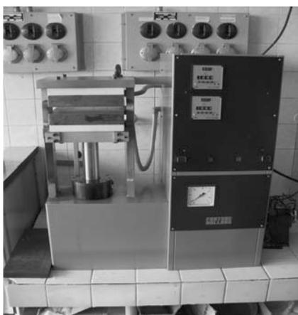
Fig. 8. Hot press for preparation of plate nanocomposite samples
