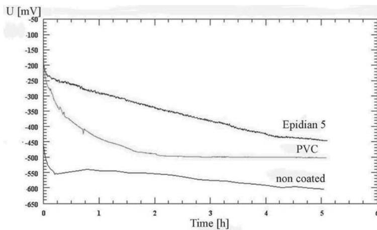
Fig. 5. Chart of measure of electrode potential of steel 45
