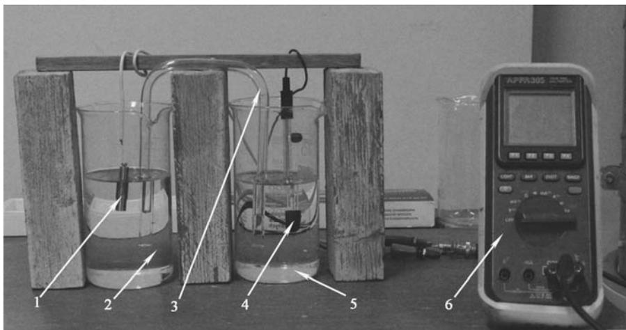
Fig. 4. View of research station: 1-Investigated sample, 2-electrolytic cell with 3% NaCl, 3-solution electrolytic bridge, 4-calomel electrode, 5-electrolytic cell with KCl saturated solution, 6-voltmeter
