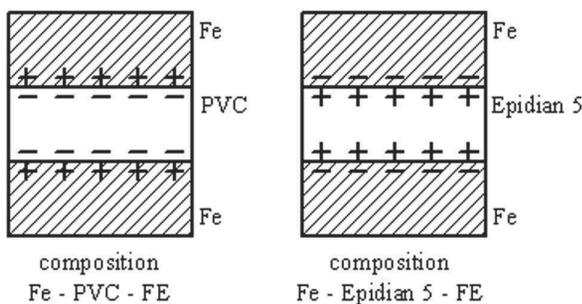
Fig. 1. Samples with EDL of negative (left) and positive polarization (right)
