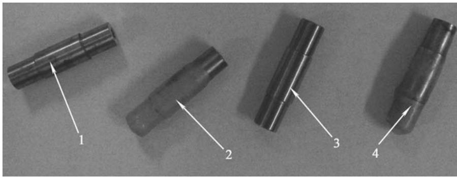
Fig. 3. Samples for tests: 1-brass M63, 2-brass M63 with coating, 3-steel 45, 4-steel 45 with coating
