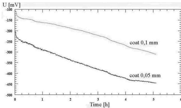
Fig. 7. Chart of measure of electrode potential of steel 45 covered with Epidian 5 with selected layer thickness
