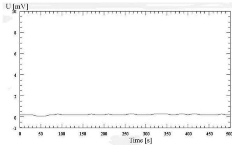
Fig. 10. Chart of measure of electrode potential of steel 45 covered with paraffin layer of 0.4 mm thickness
