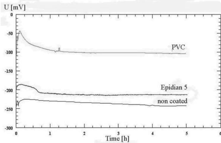
Fig. 6. Chart of measure of electrode potential of brass M63
