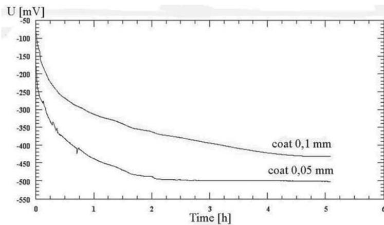
Fig. 8. Chart of measure of electrode potential of steel 45 covered with PVC with selected layer thickness
