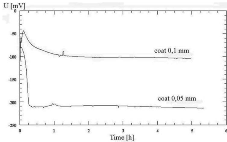
Fig. 9. Chart of measure of electrode potential of brass M63 covered with PVC with selected layer thickness
