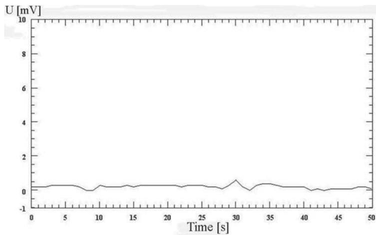
Fig. 11. Chart of electrode potential measure for brass M63 covered with paraffin layer 0.4 mm thick
