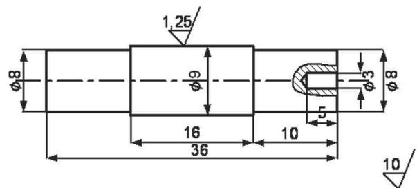
Fig. 2. Dimensions of sample for an electrode potential test
