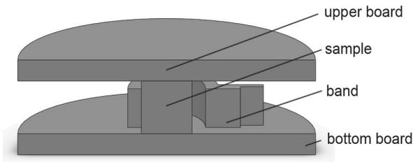
Fig. 3. The cross section image of the working part of the test stand
