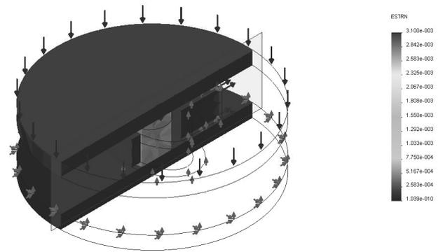
Fig. 5. The stress pattern in the analyzed tribological machine model
