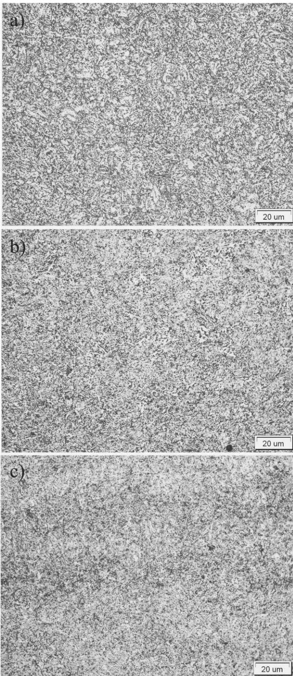
Fig. 5. High - tempered martensite in the structure of steel C45 (a), 41CrS4 (b), 42CrMoS4 (c) after quenching and tempering ( $T_{\text{austenitizing}} = 850^{\circ}\text{C}$ ,  $T_{\text{tempering}} = 580^{\circ}\text{C}$ )
