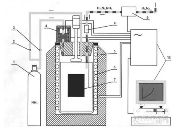
Fig. 4. A diagram of gas sulfonitriding stand: 1 - bottle of ammonia, 2 and 3 - valves regulating intensity of ammonia flow, 4 - tank of liquid sulphur, 5 - furnace, 6 - retort, 7 - sulfonitrided details, 8 - tank, 9 - control meter of ammonia dissociation degree, 10 - registration of parameters of the process [17]
