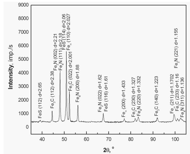
Fig. 11. Diffraction pattern of steel C45 after sulfonitriding in temperature of 570°C
