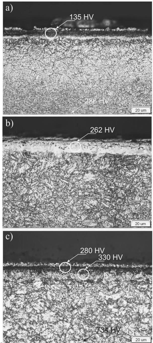
Fig. 7. Surface layer and structure of examined steel after sulfonitriding in temperature of 570°C; a - steel C45, b - steel 41CrS4, c - steel 42CrMoS4
