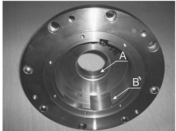
Fig. 2. A view of the flange; A - sulfonitrided surface, B' - the surface mating with the roll part B from Fig. 3
