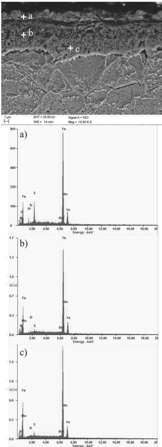
Fig. 8. Microstructure of steel C45 after sulfonitriding in temperature of 570°C and the results of chemical micro-analysis in: first zone (a), second zone (b), third zone (c) (SEM)
