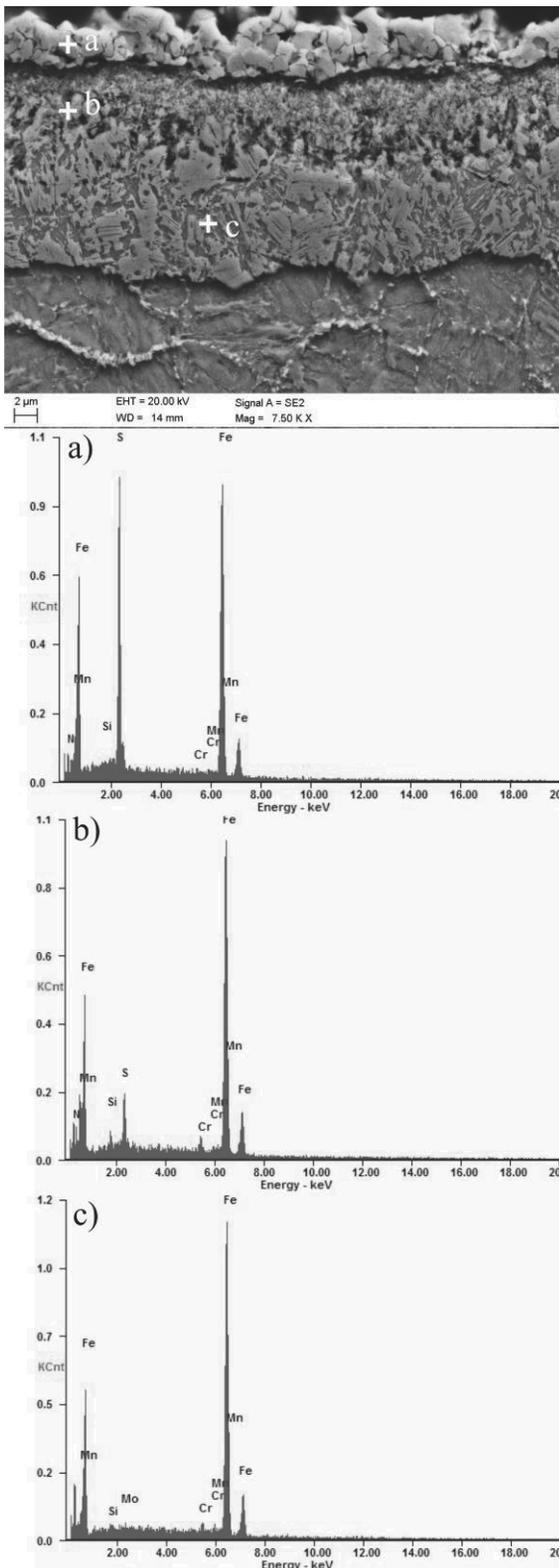
Fig. 10. Microstructure of steel 42CrMoS4 after sulfonitriding in temperature of 570°C and the results of chemical micro-analysis in: first zone (a), second zone (b), third zone (c) (SEM)
