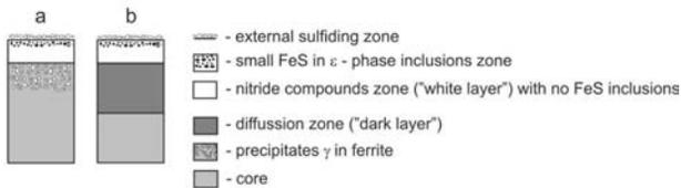
Fig. 1. Structure flowchart of surface layer on the parts after gas sulfonitriding: a - carbon steel and grey plain cast iron, b - alloy steel and alloy cast iron including nitrogen-forming elements [10]
