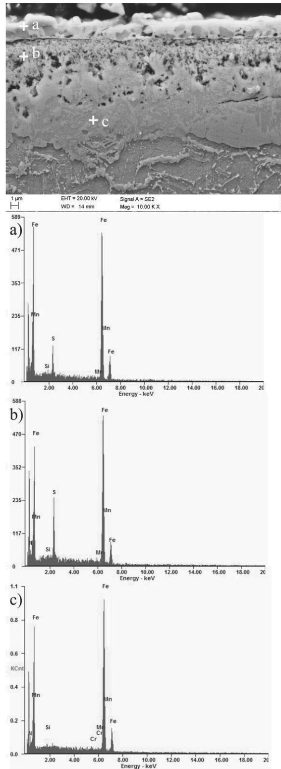
Fig. 9. Microstructure of steel 41CrS4 after sulfonitriding in temperature of 570°C and the results of chemical micro-analysis in: first zone (a), second zone (b), third zone (c) (SEM)
