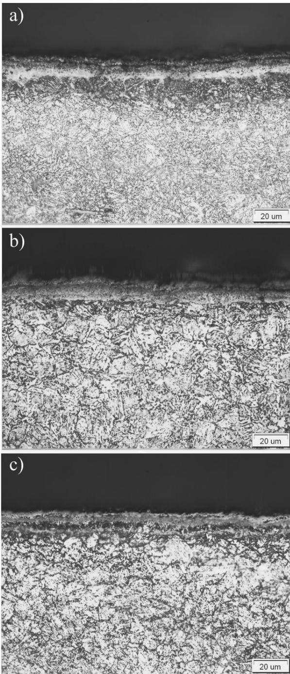
Fig. 6. Surface layer and structure of examined steel after sulfonitriding in temperature of 540°C; a - steel C45, b - steel 41CrS4, c - steel 42CrMoS4
