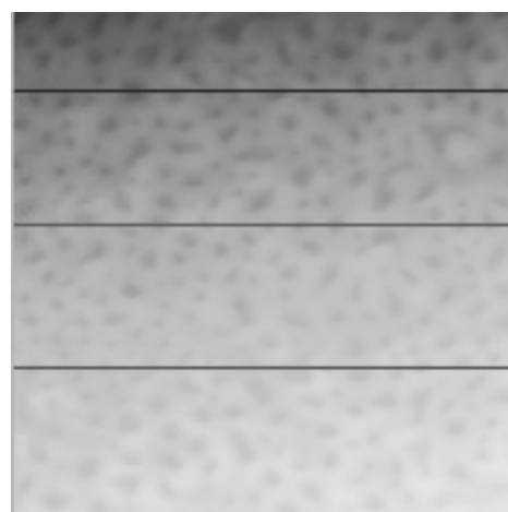
Fig. 15. Sensor image of Oxad-Si-B thin film deposited from 0.77% solution concentration with signed profiles
