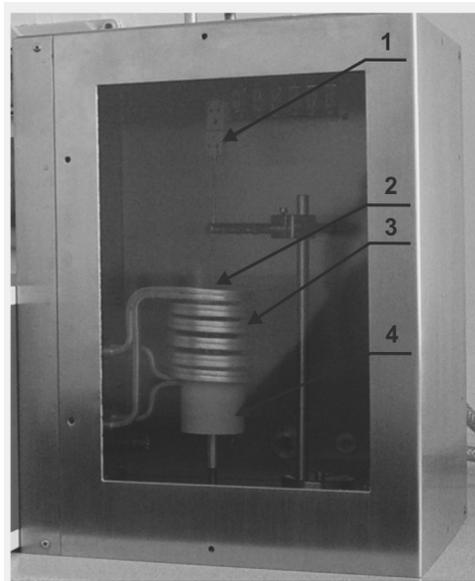
Fig. 3. Working chamber of the UMMA device: 1 – thermocouple, 2 – tested sample, 3 – induction coil, 4 – ceramic isolation
