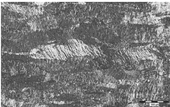
Fig. 15. Al microstructure after the 1 st pass (upright cut)
