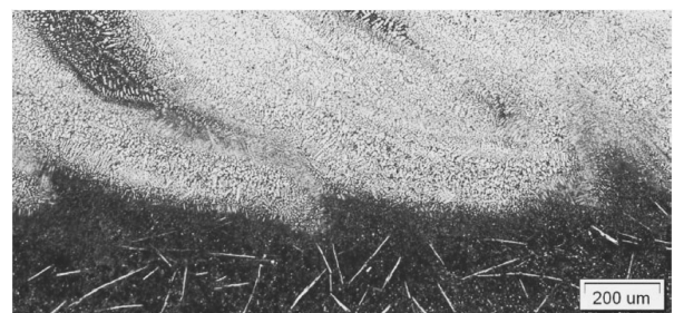
Fig. 11. Microstructure of 18GT “austenite-nano-austenite” armour plate unit: fusion line of hard nanostructural layer and soft austenite layer, magnification 100x
