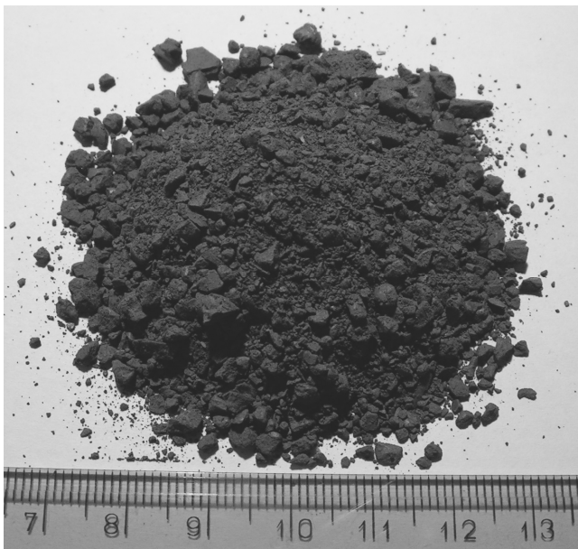
Fig. 3. The granulated feedstock after extrusion and milling
