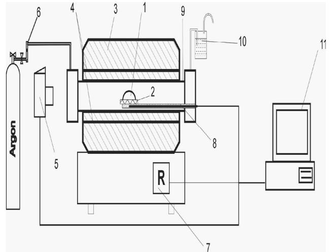
Fig. 2. Schematic view of measuring apparatus: 1 – drop of liquid metal, 2 – substrate, 3 – high temperature furnace, 4 – heating elements, 5 – CCD camera, 6 – gas delivery system, 7 – furnace work regulator, 8 – loading system with thermoelement, 9 – reactor, 10 – gas outlet system, 11 – PC computer
