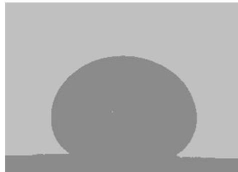
Fig. 3. An alloy drop of Cu – 0.01 X Fe at 1473 K
