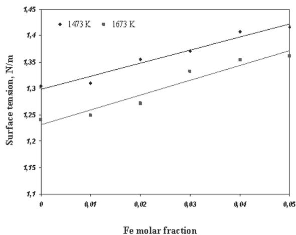
Fig. 4. Surface tension isotherms of Cu-Fe alloys at 1473 K and 1673 K
