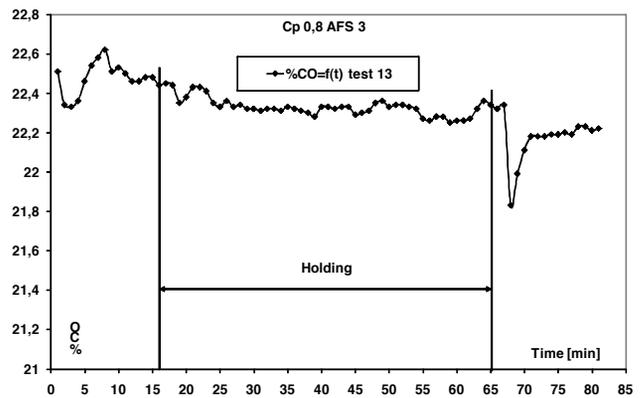
Fig. 6. Example of relation percentage content of CO in furnace atmosphere in function of time of hardening as per group No 4
