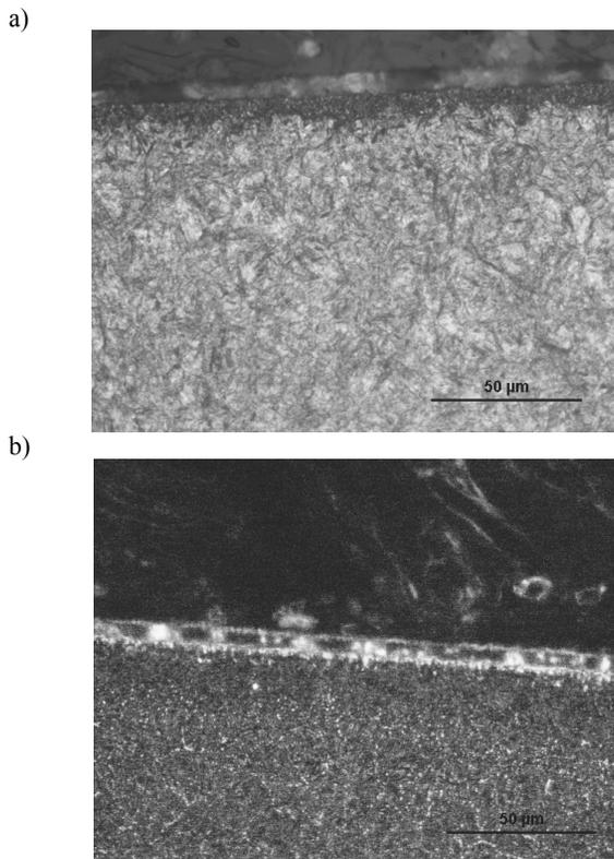
Fig. 11. (a) Example of the microstructure of carbureted layer in the area of the tip diameter of the gear with visible visible tempered martensite, (b) example of the microstructure of the carbureted layer - without the precipitate of carbides
