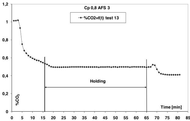
Fig. 7. Example of percentage content of CO<sub>2</sub> in furnace atmosphere in function of hardening time as per group No 4
