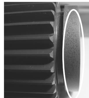
Fig. 3. Example of part with stray carb on non carburized area
