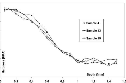
Fig. 9. Hardness chart for gear top layer after protection implementation
