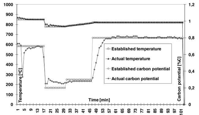
Fig. 5. Sample run of hardening process of hardening according to group No 4
