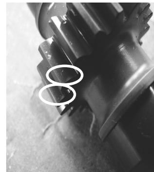
Fig. 2. Example of part with decarburized surfaces
