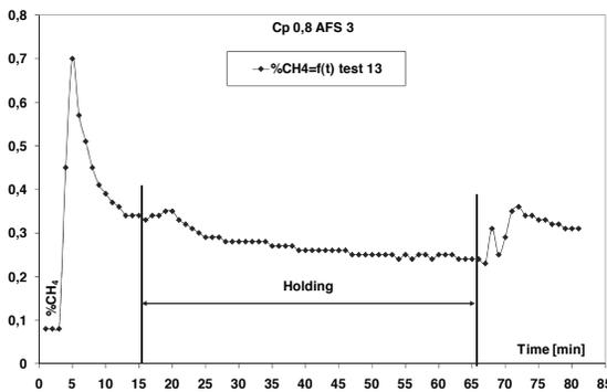
Fig. 8. Example of relation of percentage content of CH<sub>4</sub> in furnace atmosphere in function of hardening time as per group No 4
