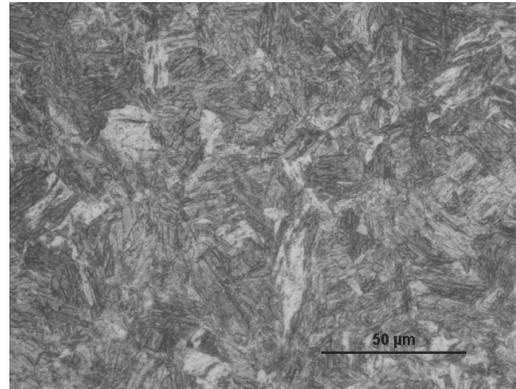
Fig. 10. Example of the core microstructure with visible tempered martensite
