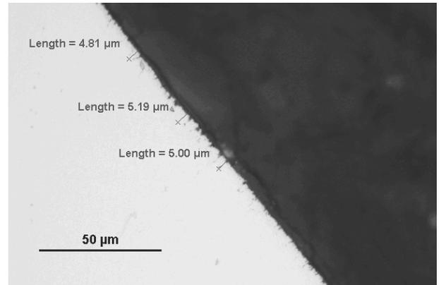
Fig. 4. Results of value of intergranular oxidation (after carburizing of the order of 0.005 mm)
