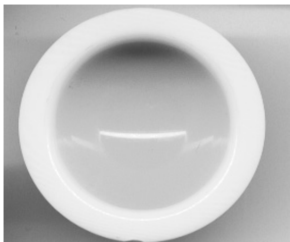
Fig. 5. The ceramic ball head Biolox ® forte (28-12/14L) before total destruction
