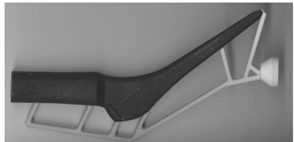
Fig. 10. The second version of model of femoral part for one employing made from black ceramic with commercial denomination (ZP150 + ZB150 Black) [21]
