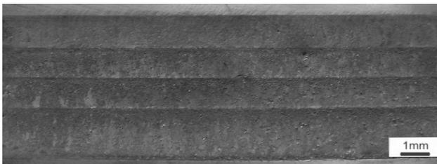
Fig. 40. View of the MCMgAl6Zn1 casting magnesium alloy face of weld after laser treatment with TiC, scan rate: 0.75 m/min, laser power: 1.6 kW
