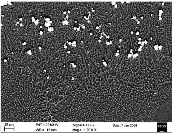
Fig. 25. Scanning electron microscope micrograph of laser modified surface of the MCMgAl6Zn1 alloy with WC particles at the interface between the modified zone and the substrate, scan rate: 0.5 m/min, laser power: 1.6 kW
