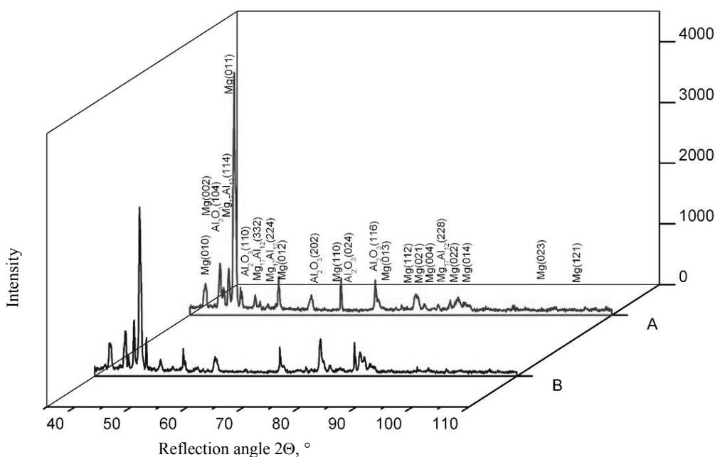
Fig. 30. X-ray diffraction pattern of MCMgAl12Zn1 casting magnesium alloys after laser treatment by aluminium oxide powder, scan rate: 0.75 m/min, laser power: A – 2.0 kW, B – 1.6 kW
