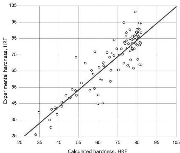
Fig. 3. Real hardness value and calculating value comparison for all test data sets
