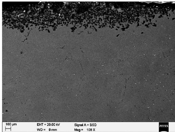
Fig. 26. Scanning electron microscope micrograph of laser modified surface layer of the MCMgAl6Zn1 alloy with SiC particles, scan rate: 0.75 m/min, laser power: 1.6 kW
