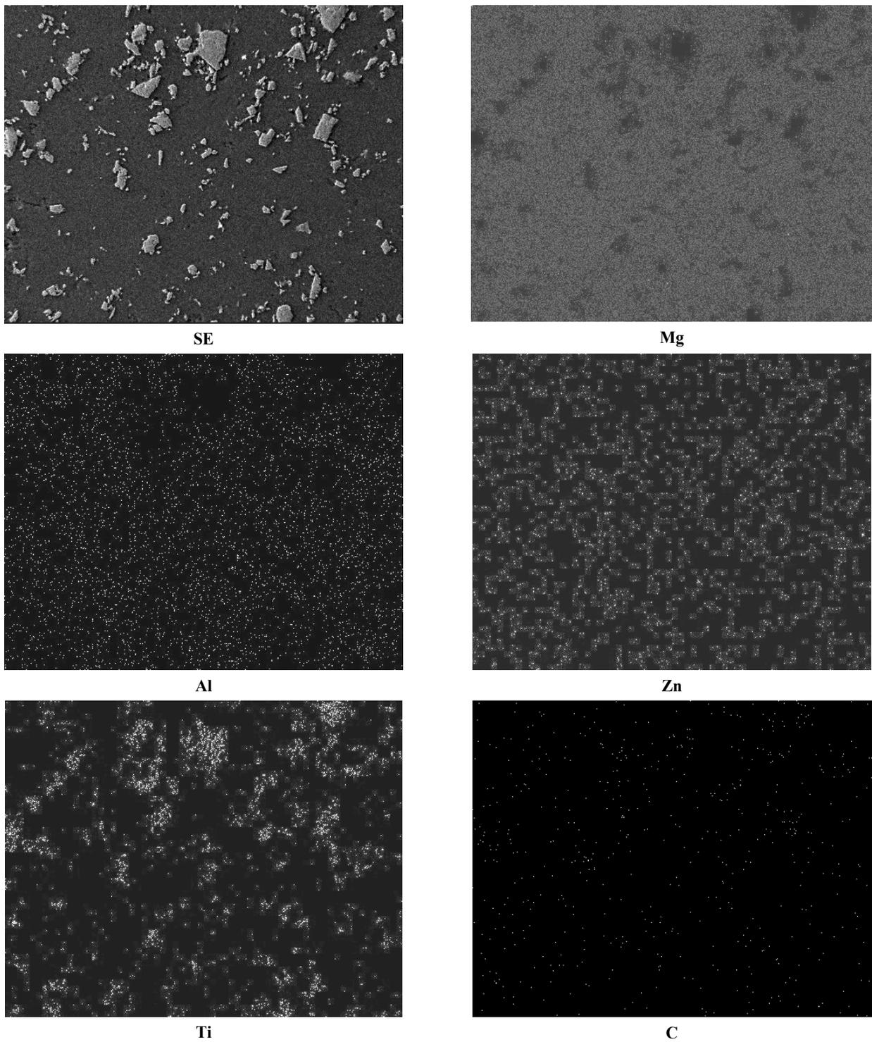
Fig. 45. X-ray mapping of the microstructure MCMgAl6Zn1 cladding layer and the distribution of Mg, Al, Zn, Ti, C, scan rate: 0.75 m/min, laser power: 1.6 kW
