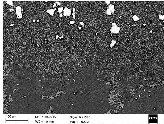
Fig. 24. Scanning electron microscope micrograph of laser modified surface of the MCMgAl9Zn1 alloy with TiC particles at the interface between the modified zone and the substrate, scan rate: 1 m/min, laser power: 1.6 kW
