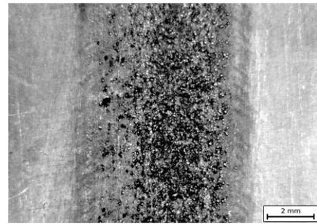
Fig. 11. View of the MCMgAl12Zn1 casting magnesium alloy face of weld after laser treatment with  $\text{Al}_2\text{O}_3$ , scan rate: 0.5 m/min, laser power: 2.0 kW
