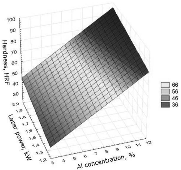
Fig. 37. Simulation of the laser power and aluminium concentration (wt.%) influence on hardness of casting magnesium alloys after laser treatment with WC particles, scan rate 0.75 m/min
