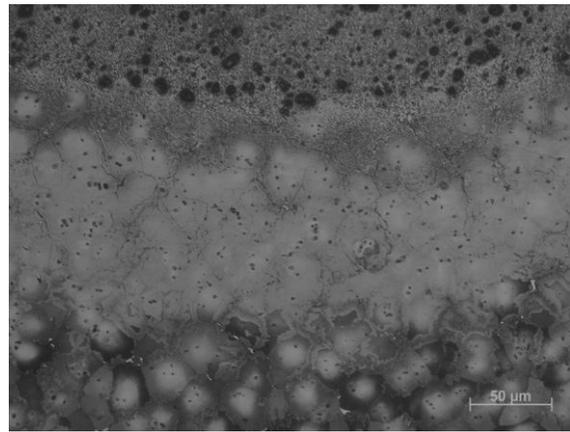
Fig. 18. Structure of the interface between the laser-melted zone, heat affected zone and the substrate of the MCMgAl12Zn1 alloy after laser treatment with WC particles, scan rate: 0.75 m/min, laser power: 2.0 kW
