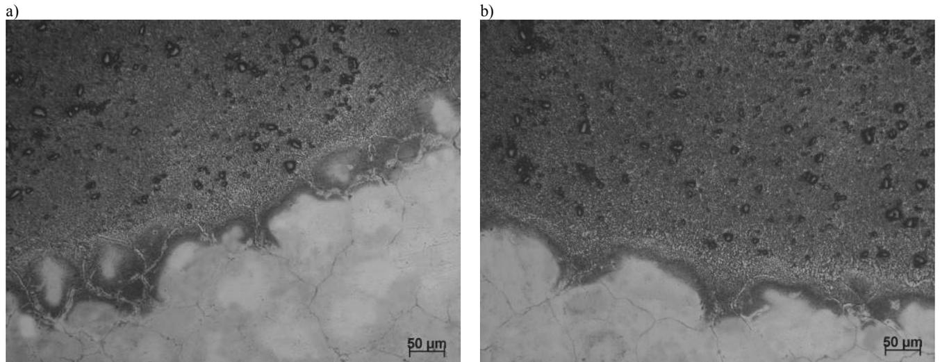
Fig. 43. Boundary between alloyed zone and heat affected zone of MCMgAl6Zn1 alloy after laser treatment with TiC particles, scan rate: 0.75 m/min, laser power: 1.6 kW
