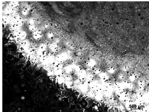
Fig. 20. Remelting path edge of the MCMgAl9Zn1 alloy surface layer after laser treatment with WC particles, scan rate: 0.75 m/min, laser power: 2.0 kW
