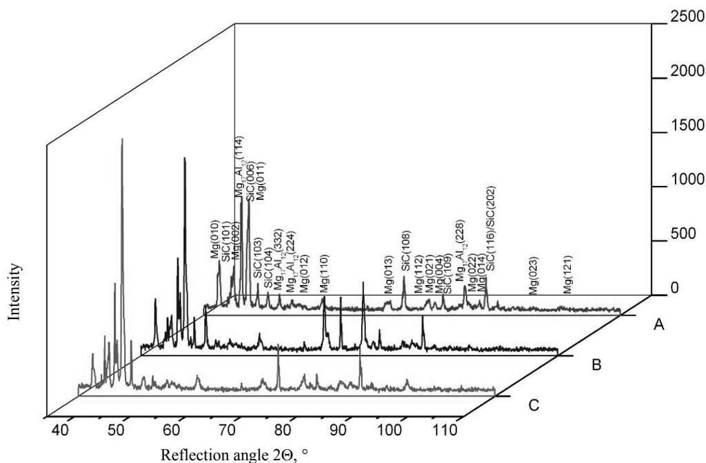
Fig. 29. X-ray diffraction pattern of MCMgAl12Zn1 casting magnesium alloys after laser treatment by silicon carbide powder, scan rate: 0.75 m/min, laser power: A – 1.2 kW, B – 1.6 kW, C – 2.0 kW
