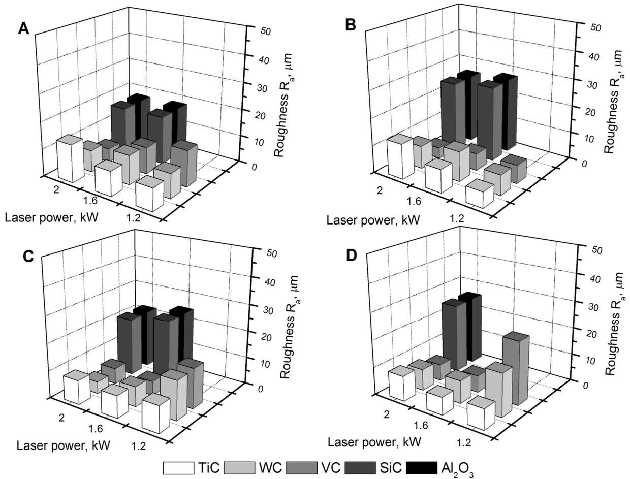
Fig. 12. Laser power and Al mass concentration influence on roughness of alloyed surface layer: A – MCMgAl3Zn1; B – MCMgAl6Zn1; C – MCMgAl9Zn1; D – MCMgAl12Zn1
