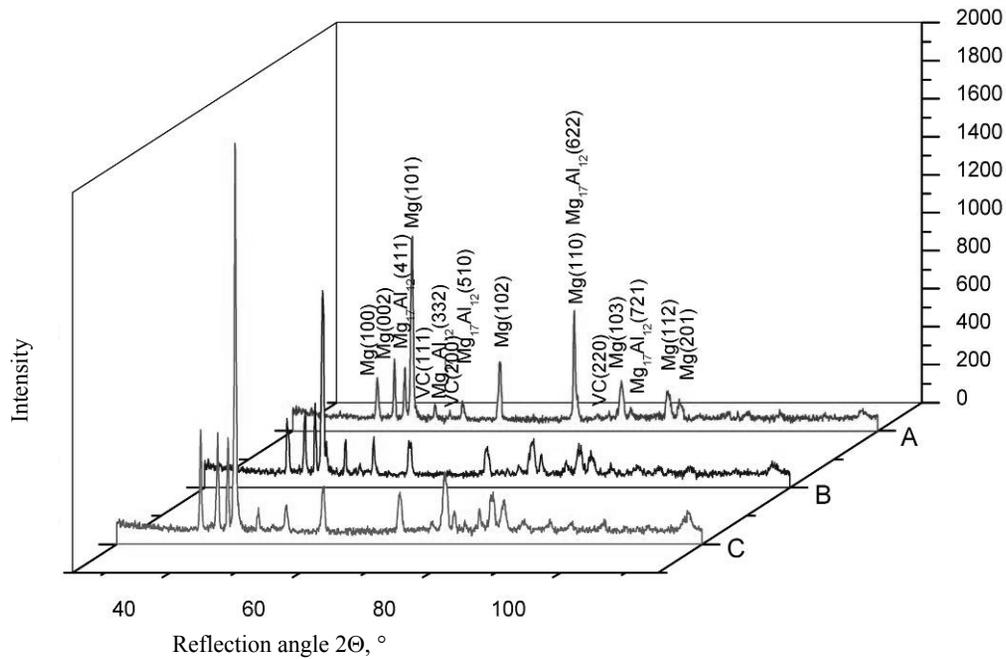
Fig. 31. X-ray diffraction pattern of MCMgAl12Zn1 casting magnesium alloys after laser treatment by vanadium carbide powder, scan rate: 0.75 m/min, laser power: A – 1.2 kW, B – 1.6 kW, C – 2.0 kW
