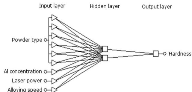
Fig. 2. Scheme of MLP neural network calculates hardness
