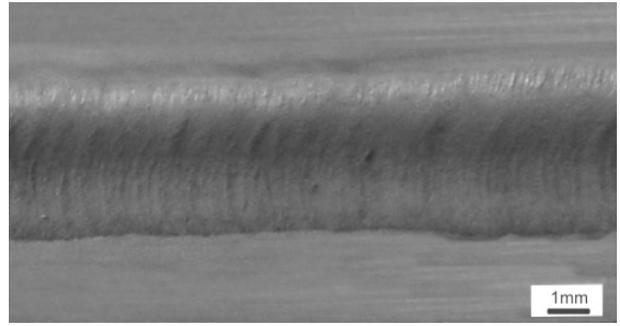
Fig. 9. View of the MCMgAl3Zn1 casting magnesium alloy face of weld after laser treatment with WC, scan rate: 0.75 m/min, laser power: 1.2 kW
