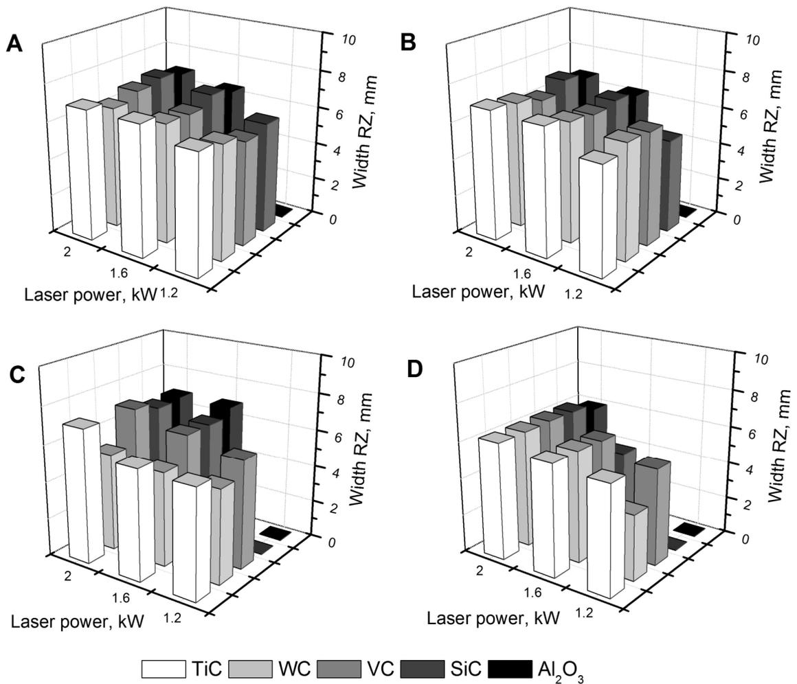
Fig. 16. Dependence of the remelting width from laser power aluminium mass concentration casting magnesium alloys after laser cladding: A – MCMgAl3Zn1, B – MCMgAl6Zn, C – MCMgAl9Zn1, D – MCMgAl12Zn1
