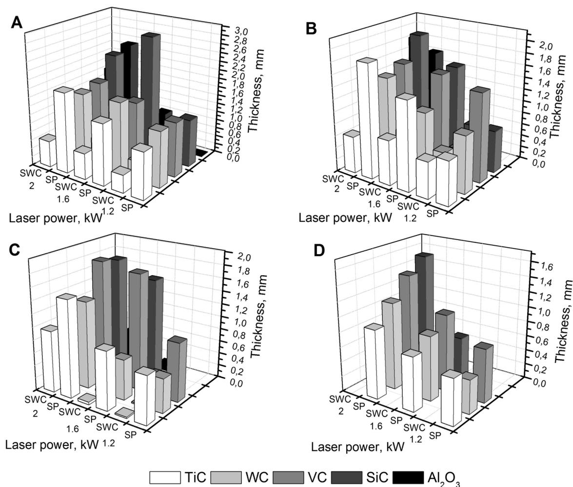
Fig. 15. Effect of laser power and the substrate material on the thickness of the SP melted zone, SWC heat affected zone and the WW surface layer of casting alloys after laser remelting: A – MCMgAl3Zn1, B – MCMgAl6Zn, C – MCMgAl9Zn1, D – MCMgAl12Zn1
