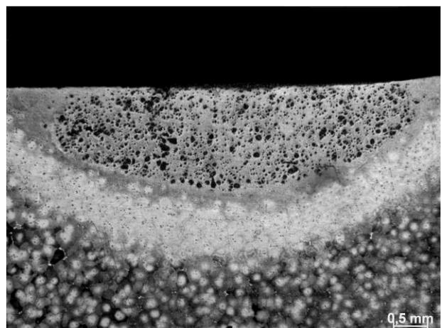
Fig. 14. Surface layer of MCMgAl9Zn1 alloy after laser treatment with WC particles, scan rate: 0.75 m/min, laser power: 2.0 kW
