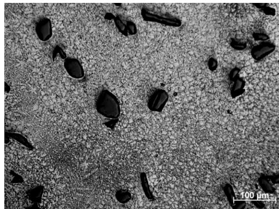
Fig. 22. Central zone of the MCMgAl6Zn1 alloy surface layer after laser treatment with SiC particles, scan rate: 0.75 m/min, laser power: 2.0 kW
