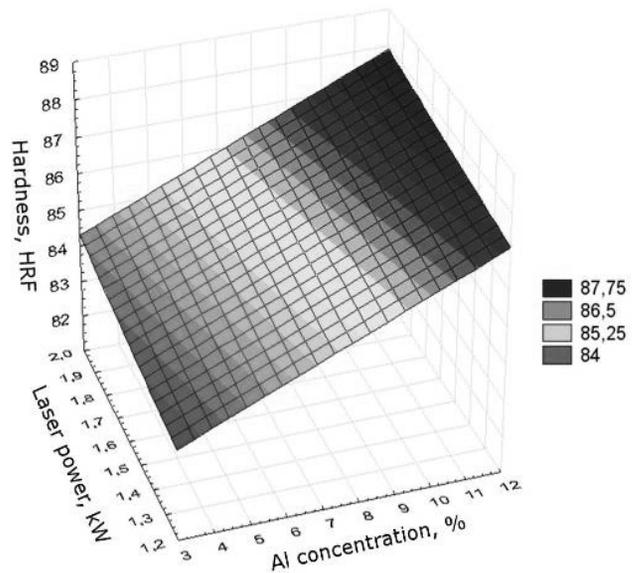
Fig. 38. Simulation of the laser power and aluminium concentration (wt.%) influence on hardness of casting magnesium alloys after laser treatment with SiC particles, scan rate 0.75 m/min
