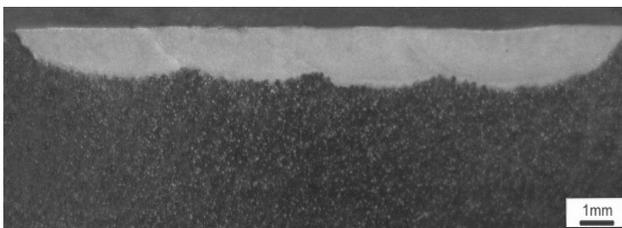
Fig. 41. Surface layer of MCMgAl6Zn1 alloy after laser treatment with TiC particles, scan rate: 0.75 m/min, laser power: 1.6 kW
