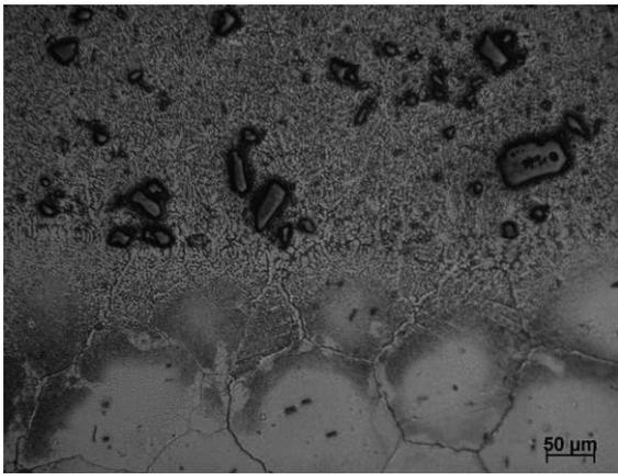
Fig. 17. Remelting path edge of the MCMgAl6Zn1 alloy surface layer after laser treatment with TiC particles, scan rate: 0.75 m/min, laser power: 1.6 kW
