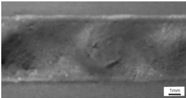
Fig. 10. View of the MCMgAl12Zn1 casting magnesium alloy face of weld after laser treatment with VC, scan rate: 0.75 m/min, laser power: 2.0 kW
