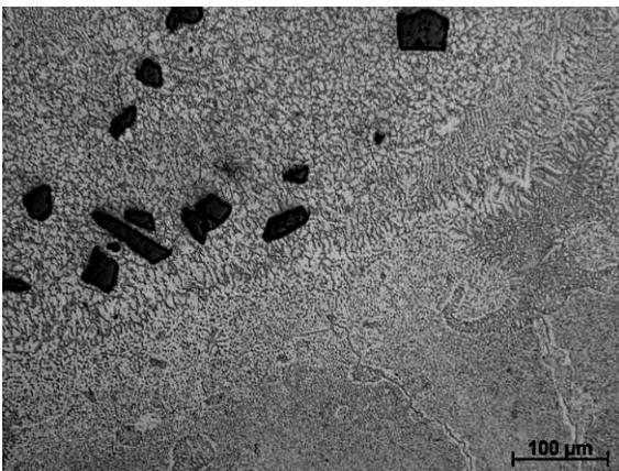
Fig. 21. Border zone of the MCMgAl12Zn1 alloy surface layer after laser treatment with SiC particles, scan rate: 0.75 m/min, laser power: 1.6 kW
