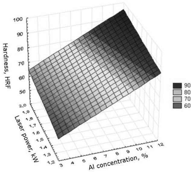
Fig. 35. Simulation of the laser power and aluminium concentration (wt.%) influence on hardness of casting magnesium alloys after laser treatment with TiC particles, scan rate 0.75 m/min
