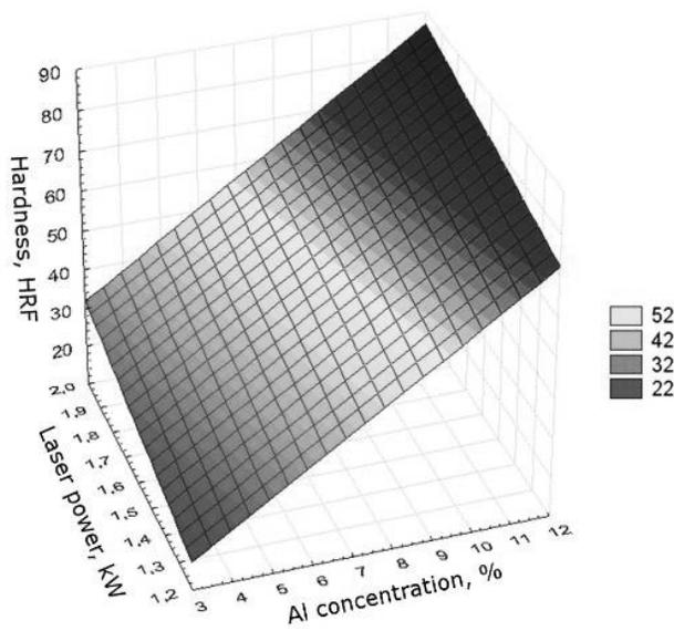
Fig. 39. Simulation of the laser power and aluminium concentration (wt. %) influence on hardness of casting magnesium alloys after laser treatment with  $Al_2O_3$  particles, scan rate 0.5 m/min
