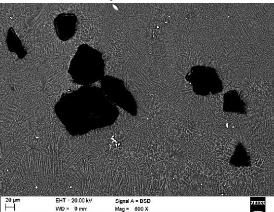
Fig. 27. Scanning electron microscope micrograph of laser modified surface of MCMgAl12Zn1 alloy with Al<sub>2</sub>O<sub>3</sub> particles of the central modified zone, scan rate: 0.5 m/min, laser power: 1.6 kW
