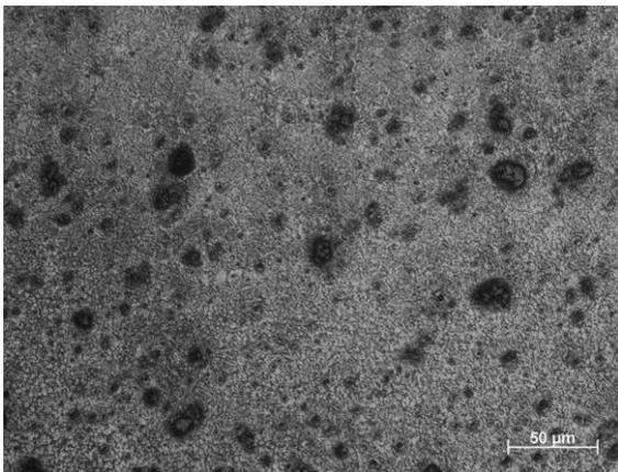
Fig. 19. Central zone of the MCMgAl12Zn1 alloy surface layer after laser treatment with WC particles, scan rate: 0.75 m/min, laser power: 2.0 kW
