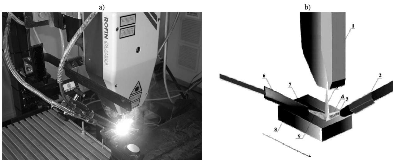
Fig. 1. a) Laser HPDL Rofin DL 020 in working process, b) Laser treatment scheme for casting magnesium alloys: 1 - laser head, 2 - transport gas cylinder and powder feed nozzle, 3 - beam laser, 4 - gas, 5 - powder, 6 - powder feed nozzle, 7 - remelting zone, 8 - base material, 9 - protective gas
