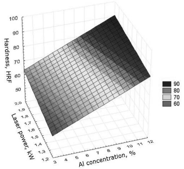
Fig. 36. Simulation of the laser power and aluminium concentration (wt.%) influence on hardness of casting magnesium alloys after laser treatment with VC particles, scan rate 0.75 m/min
