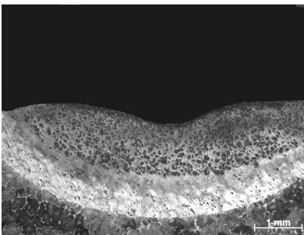
Fig. 13. Surface layer of MCMgAl12Zn1 alloy after laser treatment with TiC particles, scan rate: 0.75 m/min, laser power: 1.6 kW
