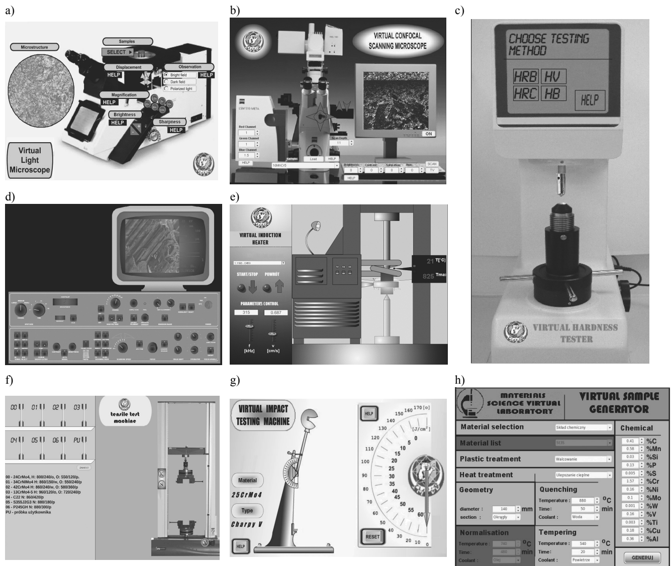
Fig. 13. Simulation of laboratory equipment installed in network material science virtual laboratory, a) light microscopy, b) laser scanning confocal microscope, c) universal hardness tester, d) scanning electron microscope, e) surface heater, f) tensile machine, g) Charpy pendulum machine, h) samples file generation panel
