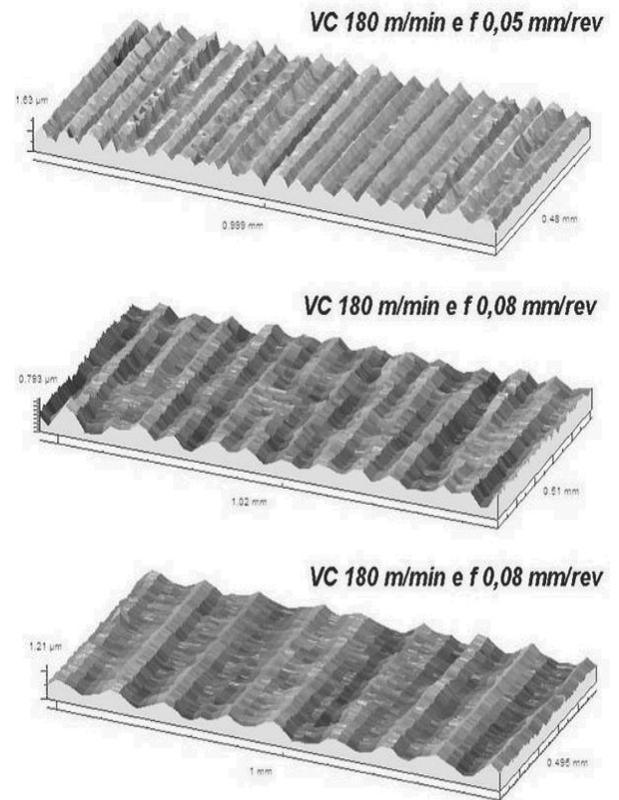
Fig. 1. Machined surface topographies with  $V_c=180$  m/min
