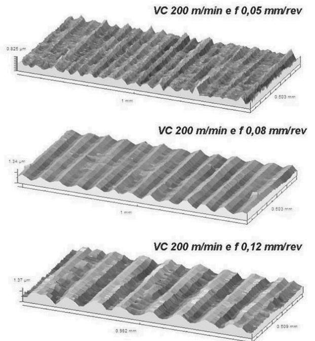
Fig. 2. Machined topographies with  $V_c=200$  m/min
