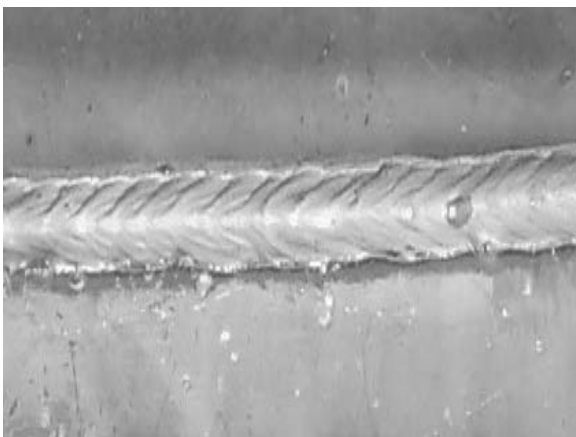
Fig. 5. Macroscopic view of the root of the weld before and after PT examination
