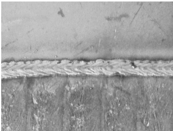
Fig. 4. Macroscopic view of the face of the weld before and after PT examination
