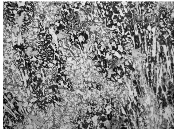
Carbides precipitations in wear resistant layer
