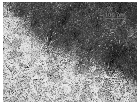
Area between weld number 2 and constructional steel
