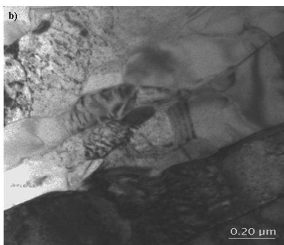
Fig. 1. Microstructure of GP91 cast steel after heat treatment (explanation in the text), a) OM; b) TEM, thin foil
