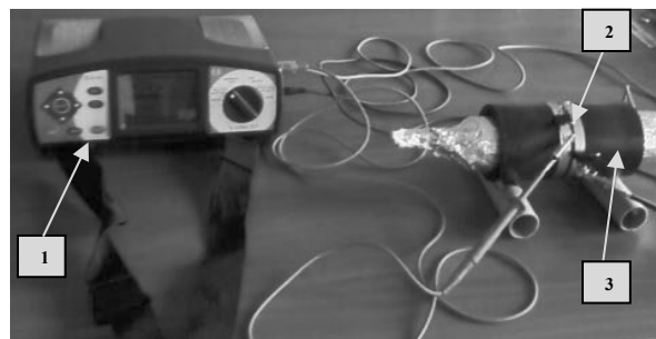
Fig. 6. System to surface resistance measurement: 1 - resistance tester, 2 - measurement electrodes, 3 - specimen
