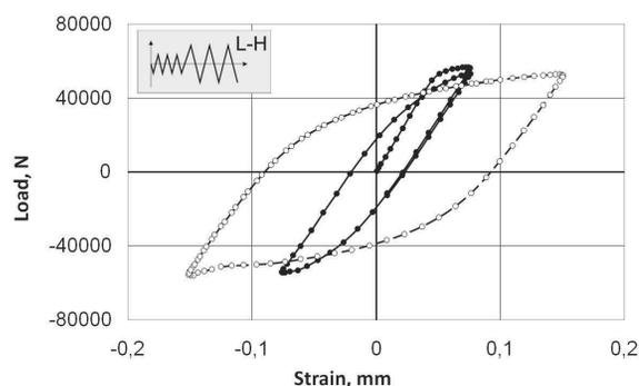
Fig. 13. Characteristic hysteresis loops recorded in test conditions of P92 steel - variant A (L-H)
