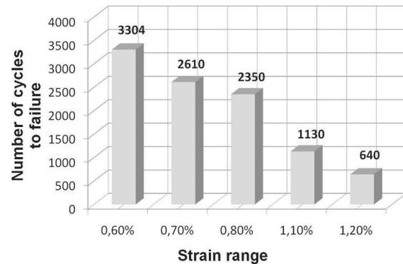
Fig. 6. Low-cycle fatigue of P92 steel
