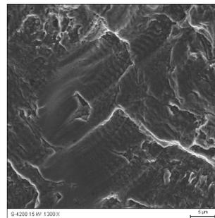
Fig. 20. Fatigue fracture of P92 steel. Distribution of fatigue striae; visible areas of fissile fracture and secondary cracks
