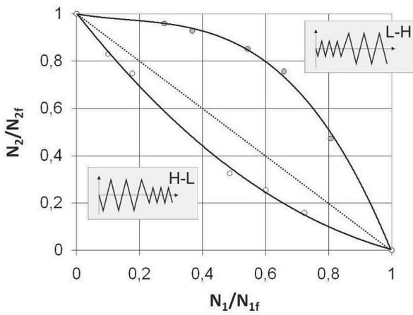
Fig. 15. Characteristics of the low-cycle fatigue durability of P91 steel under graded loads
