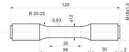
Fig. 3. Low-cycle fatigue test sample
