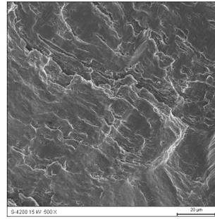
Fig. 17. Fatigue fracture of P91 steel. Distribution of resting lines in the area of transcrystalline fissile fracture
