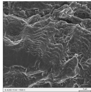
Fig. 18. Fatigue fracture of P91 steel. Distribution of fatigue striae; visible areas of fissile fracture and secondary cracks
