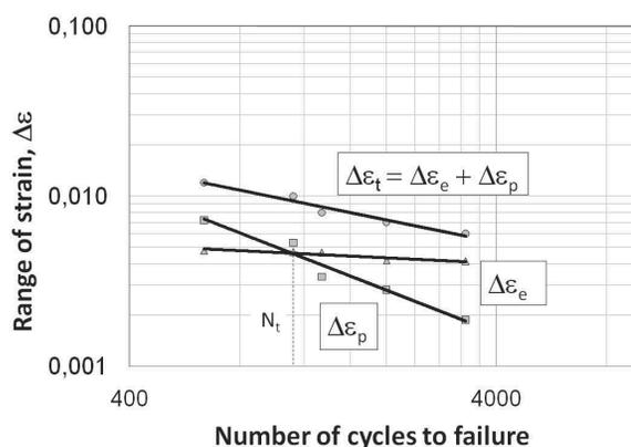
Fig. 12. Fatigue durability graphs of P92 steel
