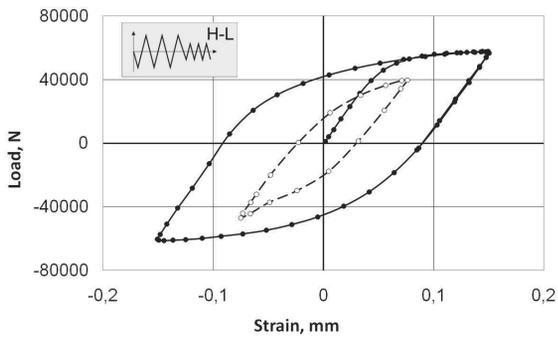
Fig. 14. Characteristic hysteresis loops recorded in test conditions of P92 steel - variant B (H-L)
