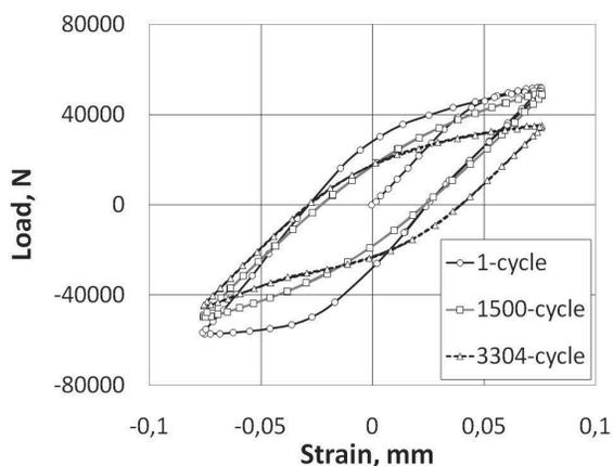
Fig. 10. Hysteresis loops recorded in  $\Delta\epsilon_t = 0,6\%$  strain range test of P92 steel
