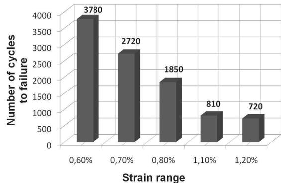
Fig. 5. Low-cycle fatigue of P91 steel
