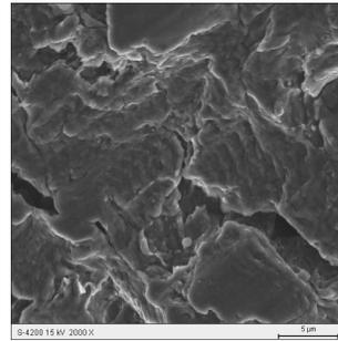
Fig. 19. Fatigue fracture of P92 steel. Distribution of fatigue striae; visible areas of fissile fracture and secondary cracks
