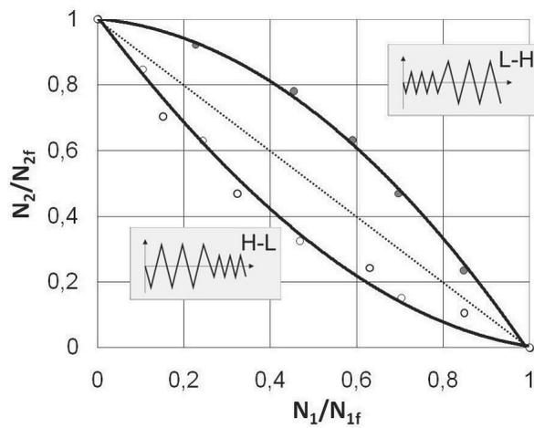
Fig. 16. Characteristics of the low-cycle fatigue durability of P92 steel under graded loads
