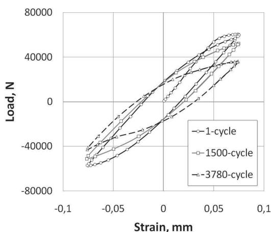
Fig. 9. Hysteresis loops recorded in  $\Delta\epsilon_t = 0,6\%$  strain range test of P91 steel
