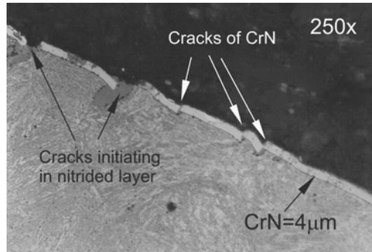
c) CrN (4 µm)/2000 forgings
