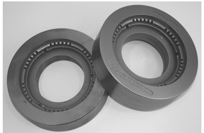
Fig. 1. Two series of dies made of DIN 1.2344 steel: (a) for production of gears pre-forging and (b) for production of steel synchronizer rings
