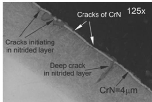
Fig. 4. The analysis of the failure intensity of forging dies with nitrided layer / CrN coating composite layers after their various maintenance time
