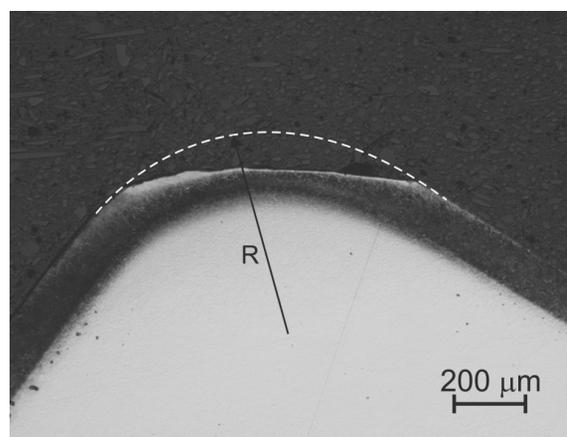
Fig. 8. The results of metallographic investigations for the die coated with a “nitrided layer/ CrN coating” layered composite after forging 2000 of steel synchronizer rings
