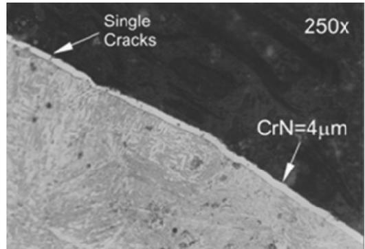
b) CrN (4 µm)/1000 forgings
