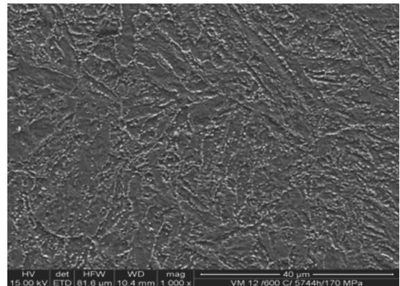
Fig. 17. Structure of the VM12(X12CrCoWVNb12-2-2) steel subjected to annealing at the temperature of 600°C over the time of 5744 h and stress of 170 MPa observed in the SEM (1000x)
