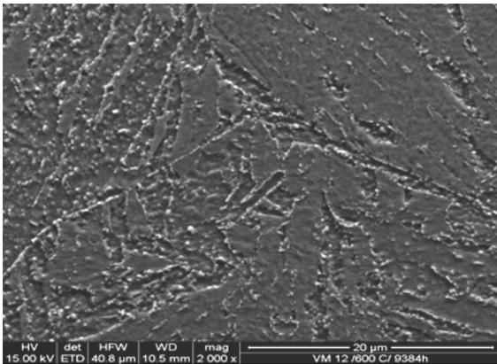
Fig. 4. Structure of the VM12(X12CrCoWVNb12-2-2) steel subjected to annealing at the temperature of 600°C over the time of 5744 h observed in the SEM (2000x)
