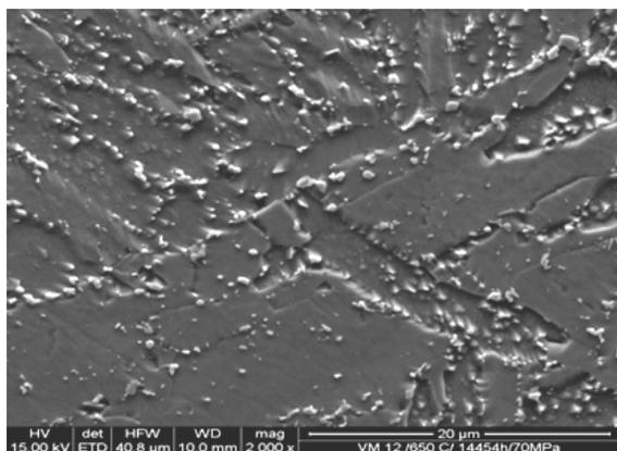
Fig. 28. Structure of the VM12(X12CrCoWVNb12-2-2) steel subjected to annealing at the temperature of 650°C over the time of 14454 h and stress of 70 MPa observed in the SEM (2000x)
