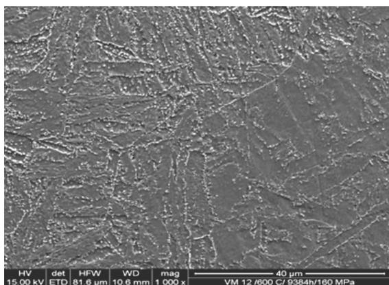
Fig. 19. Structure of the VM12(X12CrCoWVNb12-2-2) steel subjected to annealing at the temperature of 600°C over the time of 9384 h and stress of 160 MPa observed in the SEM (1000x)
