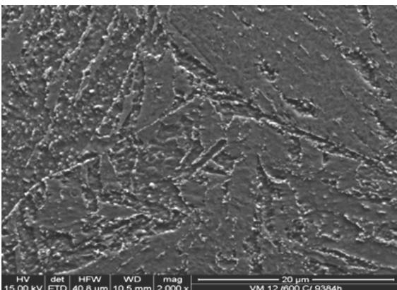
Fig. 5. Structure of the VM12(X12CrCoWVNb12-2-2) steel subjected to annealing at the temperature of 600°C over the time of 9384 h observed in the SEM (1000x)
