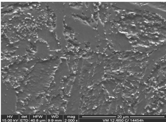
Fig. 16. Structure of the VM12(X12CrCoWVNb12-2-2) steel subjected to annealing at the temperature of 650°C over the time of 14454 h observed in the SEM (2000x)
