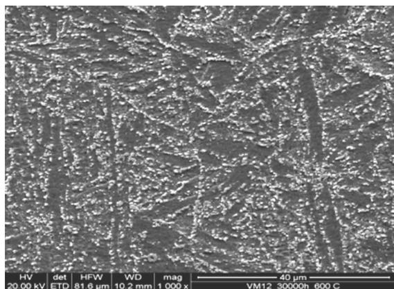
Fig. 9. Structure of the VM12(X12CrCoWVNb12-2-2) steel subjected to annealing at the temperature of 600°C over the time of 30000 h observed in the SEM (1000x)
