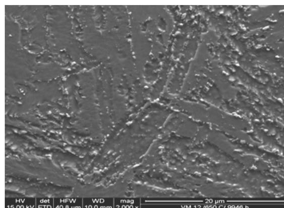
Fig. 14. Structure of the VM12(X12CrCoWVNb12-2-2) steel subjected to annealing at the temperature of 650°C over the time of 9946 h observed in the SEM (2000x)
