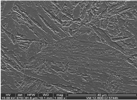
Fig. 3. Structure of the VM12(X12CrCoWVNb12-2-2) steel subjected to annealing at the temperature of 600°C over the time of 5744 h observed in the SEM (1000x)
