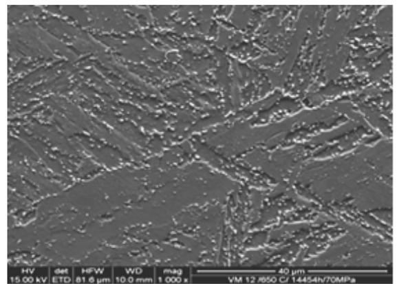
Fig. 27. Structure of the VM12(X12CrCoWVNb12-2-2) steel subjected to annealing at the temperature of 650°C over the time of 14454 h and stress of 70 MPa observed in the SEM (1000x)
