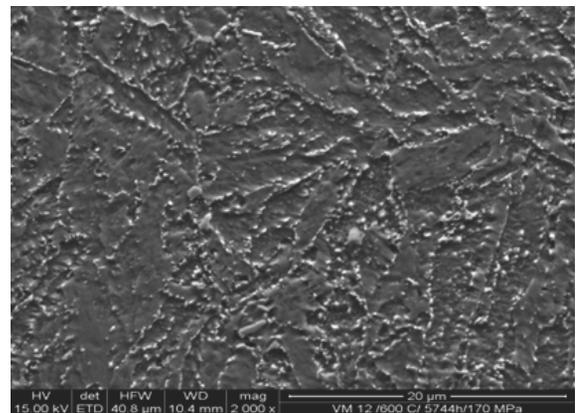
Fig. 18. Structure of the VM12(X12CrCoWVNb12-2-2) steel subjected to annealing at the temperature of 600°C over the time of 5744 h and stress of 170 MPa observed in the SEM (2000x)
