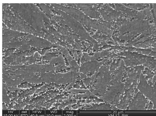
Fig. 2. Structure of the VM12(X12CrCoWVNb12-2-2) steel observed in the SEM (2000x)
