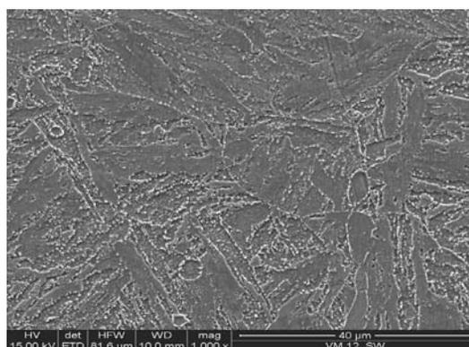
Fig. 1. Structure of the VM12(X12CrCoWVNb12-2-2) steel observed in the SEM (1000x)
