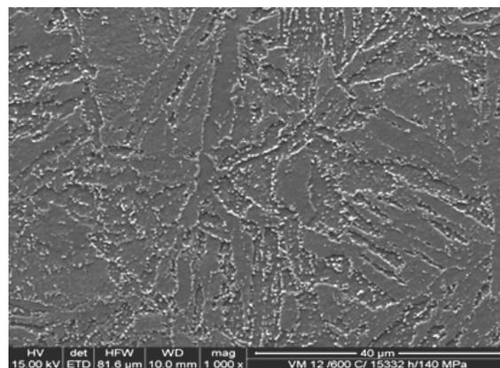
Fig. 21. Structure of the VM12(X12CrCoWVNb12-2-2) steel subjected to annealing at the temperature of 600°C over the time of 15322 h and stress of 140 MPa observed in the SEM (1000x)
