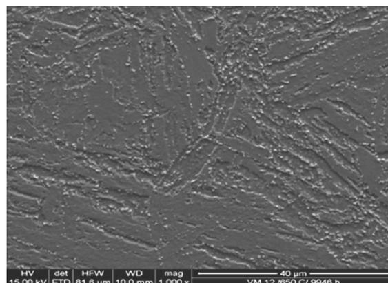
Fig. 13. Structure of the VM12(X12CrCoWVNb12-2-2) steel subjected to annealing at the temperature of 650°C over the time of 9946 h observed in the SEM (1000x)
