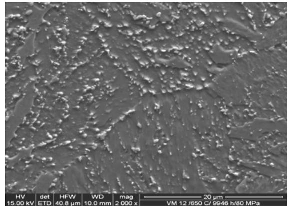
Fig. 26. Structure of the VM12(X12CrCoWVNb12-2-2) steel subjected to annealing at the temperature of 650°C over the time of 9946 h and stress of 80 MPa observed in the SEM (2000x)
