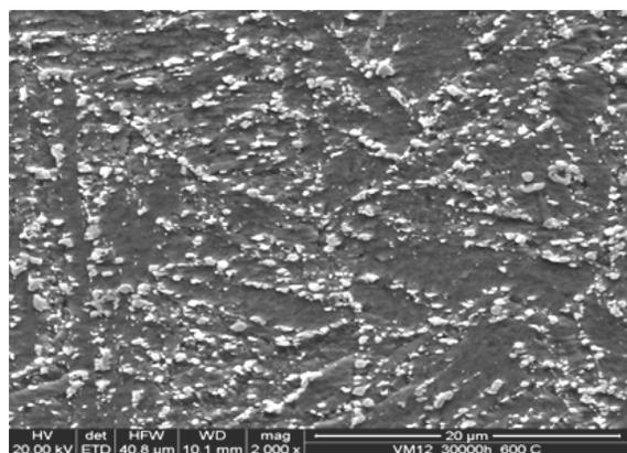
Fig. 10. Structure of the VM12(X12CrCoWVNb12-2-2) steel subjected to annealing at the temperature of 600°C over the time of 30000 h observed in the SEM (2000x)
