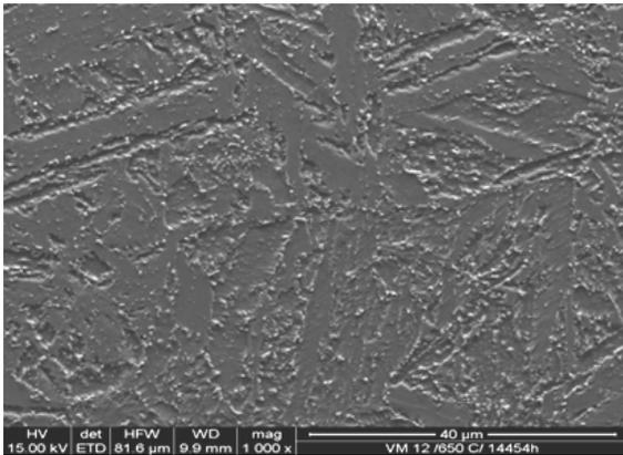
Fig. 15. Structure of the VM12(X12CrCoWVNb12-2-2) steel subjected to annealing at the temperature of 650°C over the time of 14454 h observed in the SEM (1000x)
