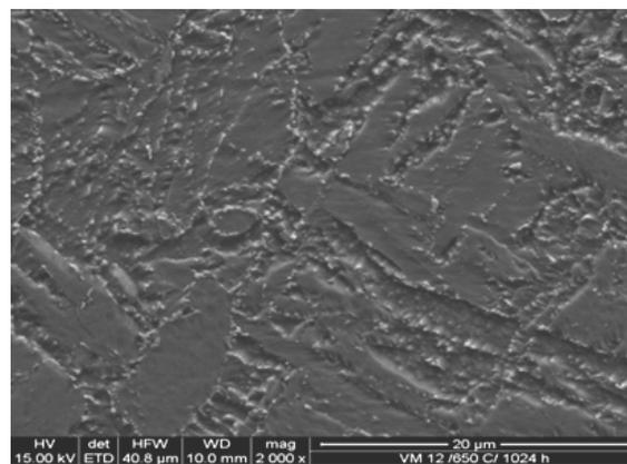
Fig. 12. Structure of the VM12(X12CrCoWVNb12-2-2) steel subjected to annealing at the temperature of 650°C over the time of 1024 h observed in the SEM (2000x)
