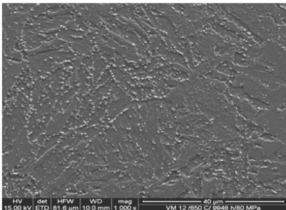
Fig. 25. Structure of the VM12(X12CrCoWVNb12-2-2) steel subjected to annealing at the temperature of 650°C over the time of 9946 h and stress of 80 MPa observed in the SEM (1000x)
