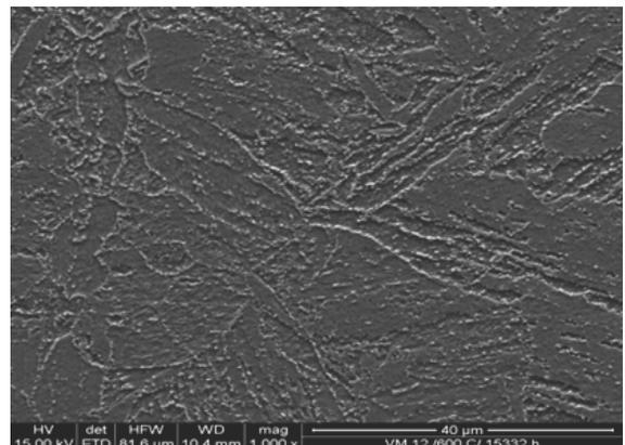
Fig. 7. Structure of the VM12(X12CrCoWVNb12-2-2) steel subjected to annealing at the temperature of 600°C over the time of 15332 h observed in the SEM (1000x)
