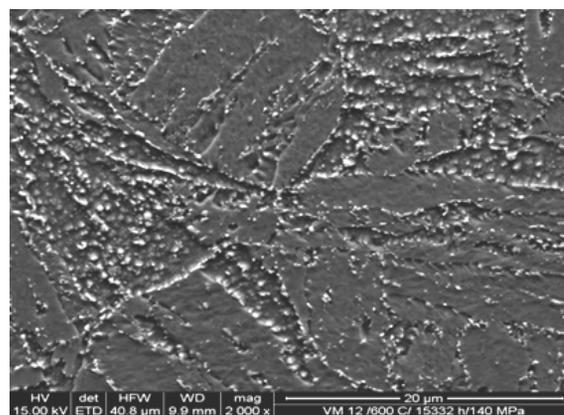
Fig. 22. Structure of the VM12(X12CrCoWVNb12-2-2) steel subjected to annealing at the temperature of 600°C over the time of 15322 h and stress of 140 MPa observed in the SEM (2000x)
