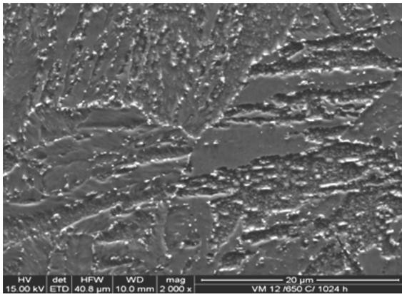
Fig. 24. Structure of the VM12(X12CrCoWVNb12-2-2) steel subjected to annealing at the temperature of 650°C over the time of 1024 h and stress of 125 MPa observed in the SEM (2000x)
