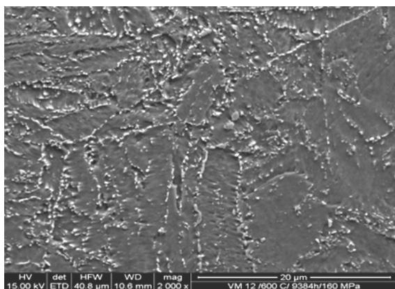
Fig. 20. Structure of the VM12(X12CrCoWVNb12-2-2) steel subjected to annealing at the temperature of 600°C over the time of 9384 h and stress of 160 MPa observed in the SEM (2000x)
