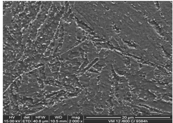
Fig. 6. Structure of the VM12(X12CrCoWVNb12-2-2) steel subjected to annealing at the temperature of 600°C over the time of 9384 h observed in SEM (2000x)
