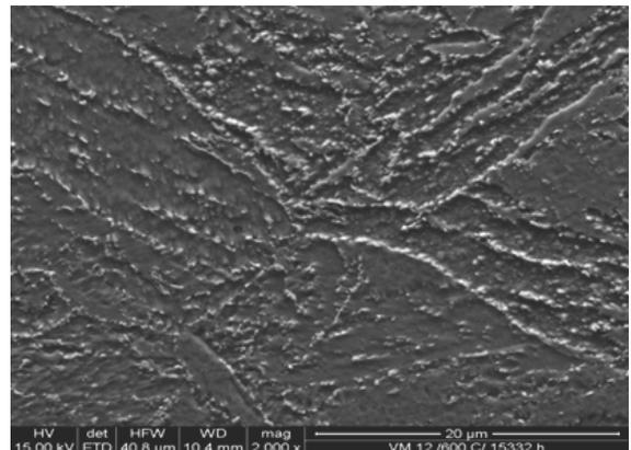
Fig. 8. Structure of the VM12(X12CrCoWVNb12-2-2) steel subjected to annealing at the temperature of 600°C over the time of 15332 h observed in the SEM (2000x)
