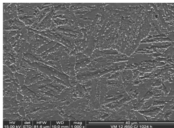
Fig. 23. Structure of the VM12(X12CrCoWVNb12-2-2) steel subjected to annealing at the temperature of 650°C over the time of 1024 h and stress of 125 MPa observed in the SEM (1000x)
