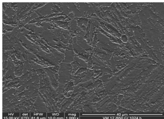
Fig. 11. Structure of the VM12(X12CrCoWVNb12-2-2) steel subjected to annealing at the temperature of 650°C over the time of 1024 h observed in the SEM (1000x)
