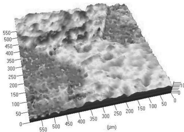
Fig. 5. CLSM three-dimensional topography of the textured wafer surface in 40% KOH:IPA:DIH<sub>2</sub>O solution
