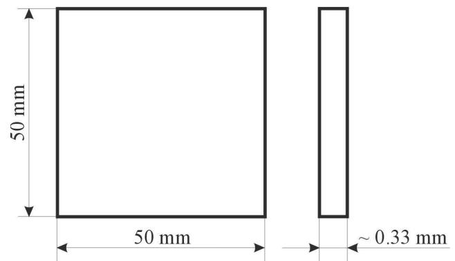
Fig. 2. Silicon wafer shape and dimensions
