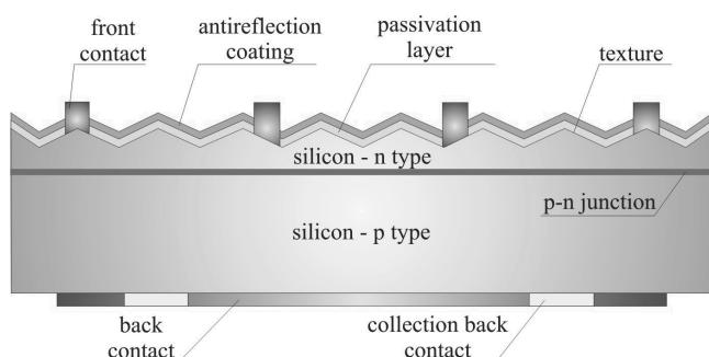
Fig. 3. Production scheme of polycrystalline silicon solar cells
