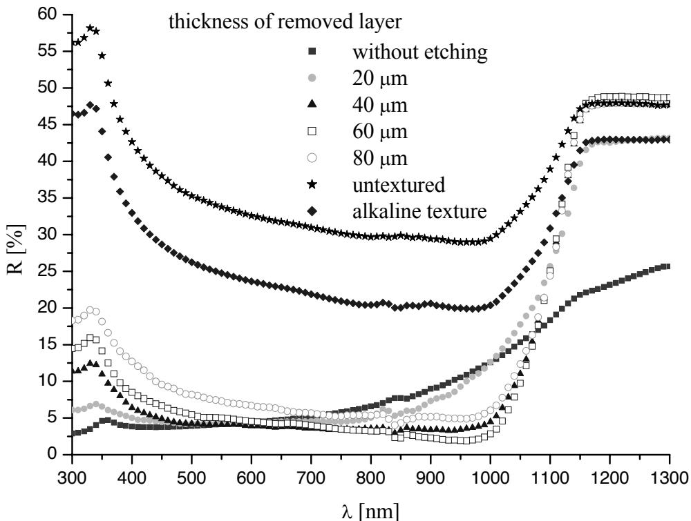
Fig. 8. The light reflection coefficient for the following polycrystalline silicon wafers: untextured, alkaline-textured, unetched laser-textured and laser-textured ones with varied thickness of layers removed during chemical etching
