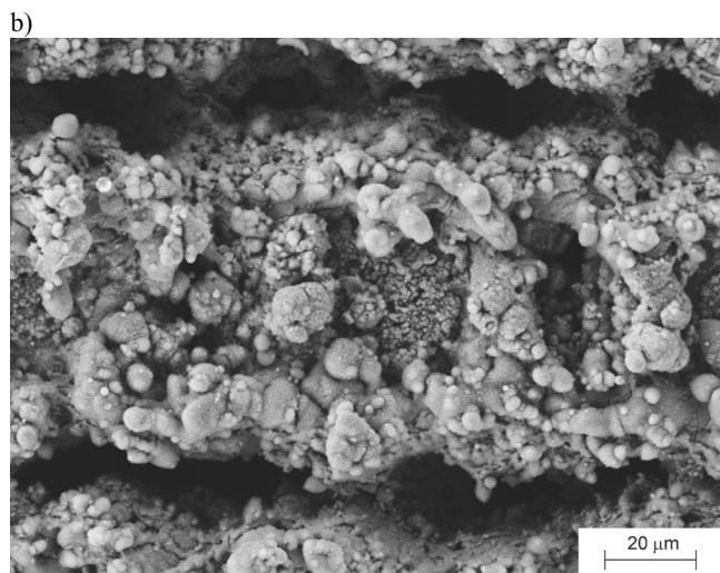
Fig. 6. SEM topography of the laser textured surface of polycrystalline silicon: a) x 150, b) x 2000
