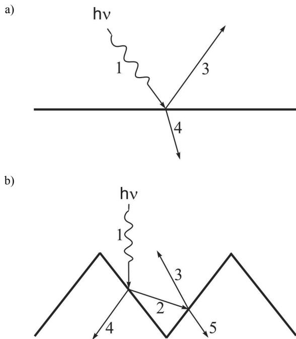
Fig. 1. The impact of surface texturing on radiation absorption: a) flat surface, b) textured surface; where: 1 – incident photon, 2, 3 – reflected photons, 4, 5 – absorbed photons
