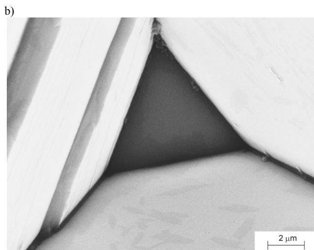
Fig. 7. SEM topography of the laser textured surface after removing 80 μm of the removed layer: a) x 150, b) x 20 000
