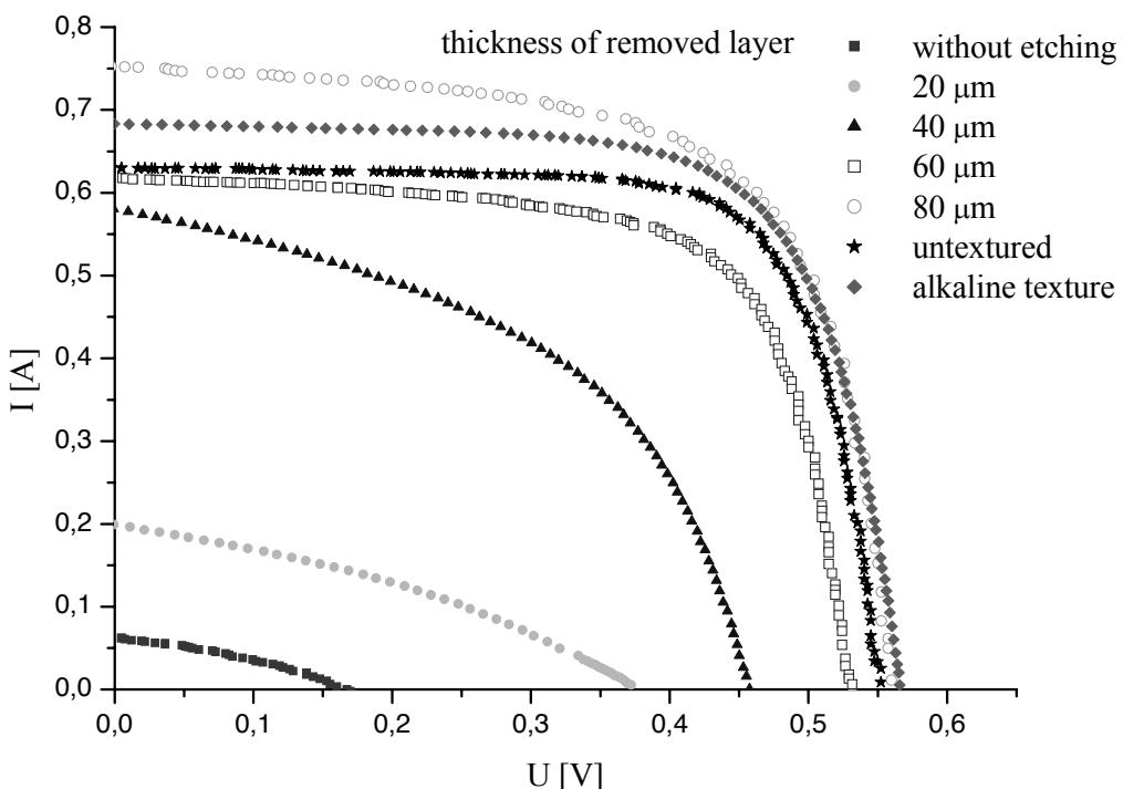
Fig. 9. The voltage-current characteristics of photovoltaic cells made of the following polycrystalline silicon wafers: untextured, alkaline textured, unetched laser-textured and laser-textured ones with varied thickness of layers removed during chemical etching
